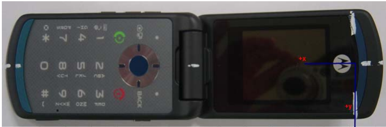
Figure 5. Coordinate Axis for T-coil Measurements
