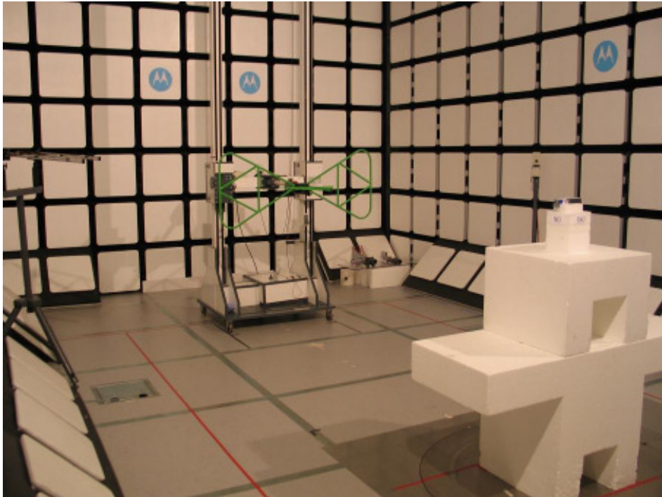
22282-1, IHDP56JM2 setup in semi-anechoic chamber – left side
