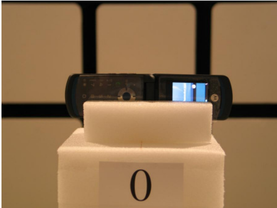
22299-1, IHDP56JM1 placed in test position Y - Open
