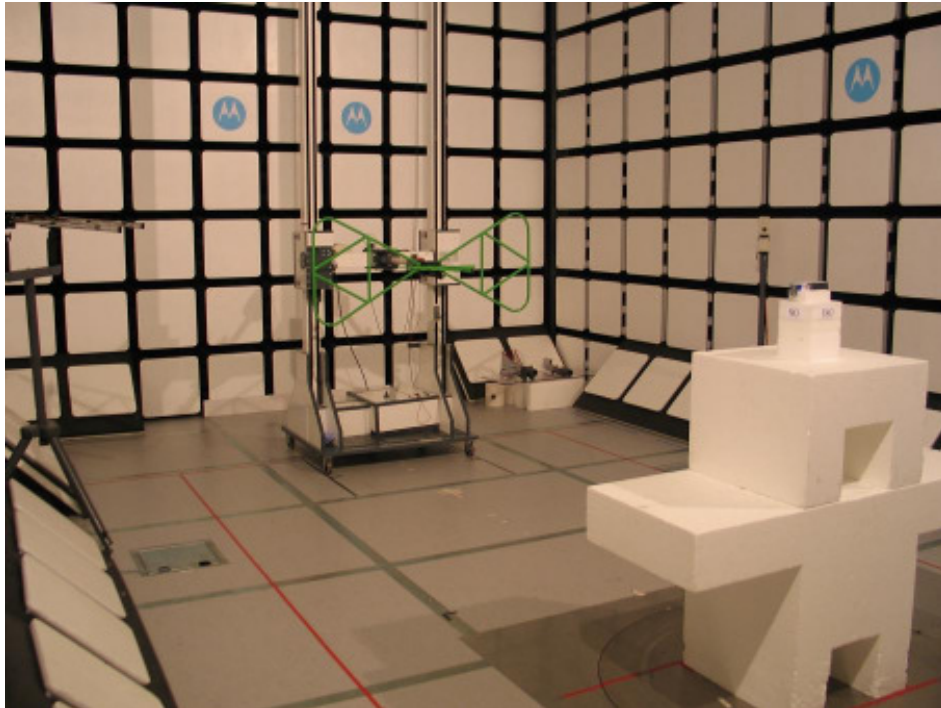
22299-1, IHDP56JM1 setup in semi-anechoic chamber – left side
