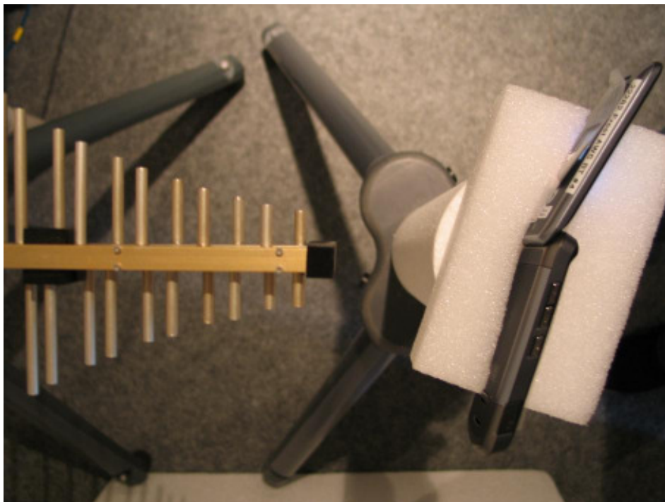
22299-1, IHDP56JM1 Check for maximum radiation at position X – Open
