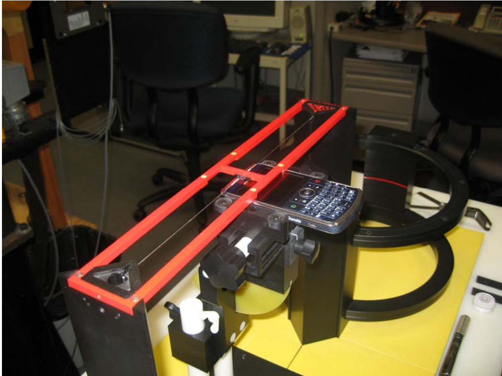
Figure 3. Positioning and Measurement for RF Emissions
