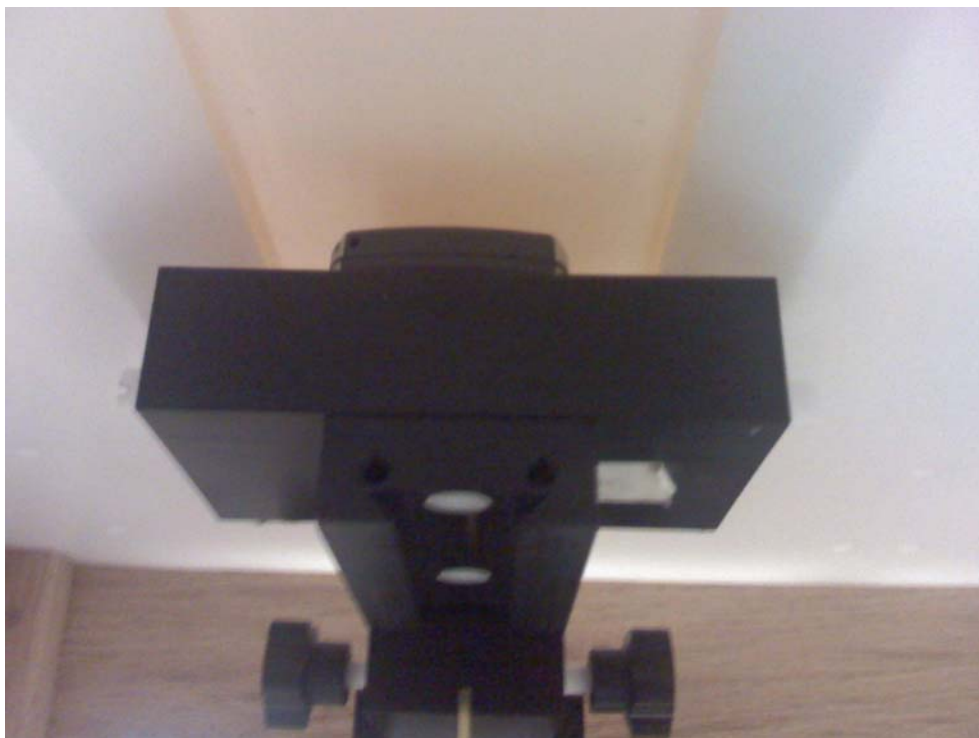
Figure 8 - Transceiver against body, 25 mm from Phantom position
