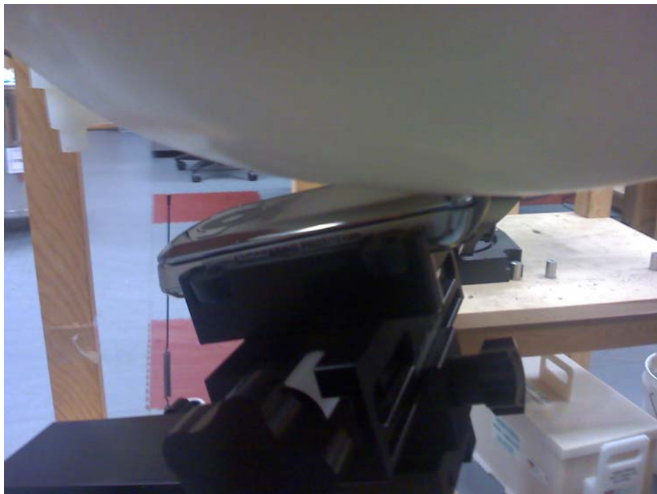
Figure 6 - Transceiver against head, 15° Tilt position – Slider Closed
