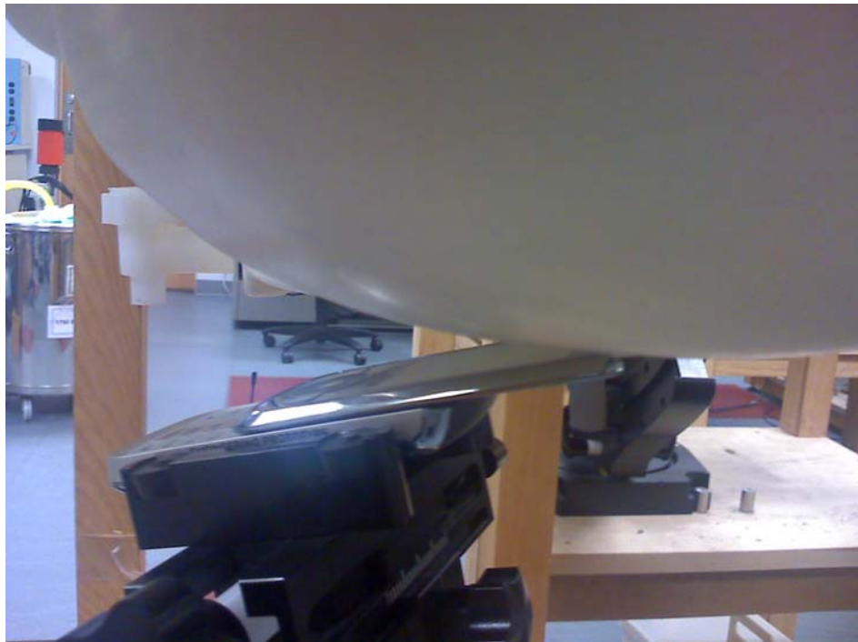
Figure 7 - Transceiver against head, 15° Tilt position – Slider Open
