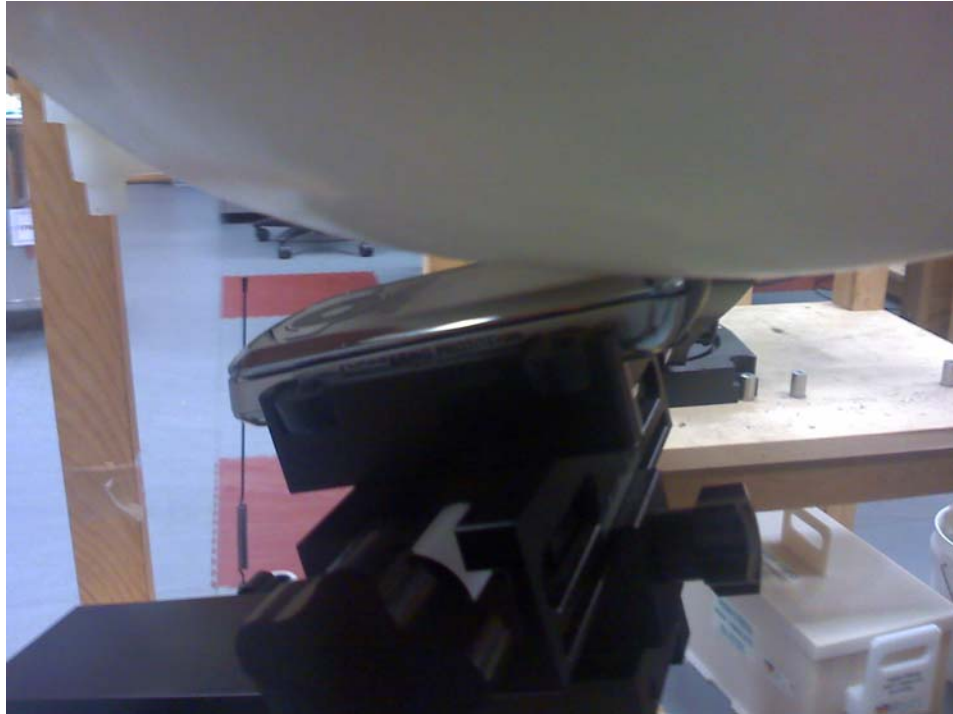
Figure 6 - Transceiver against head, 15° Tilt position – Slider Closed
