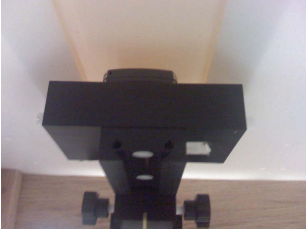
Figure 8 - Transceiver against body, 25 mm from Phantom position
