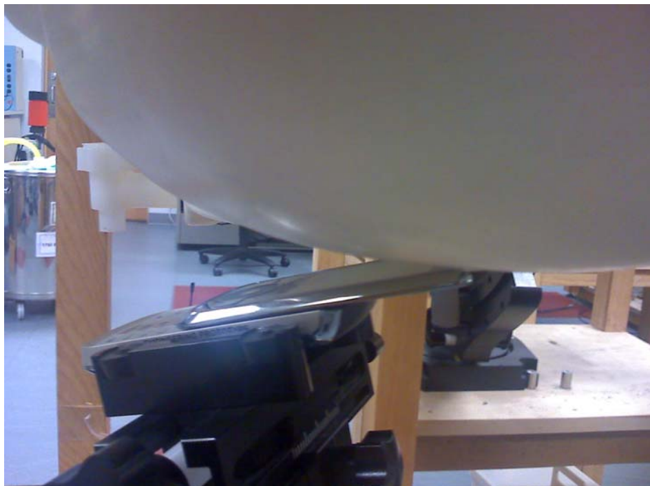
Figure 7 - Transceiver against head, 15° Tilt position – Slider Open
