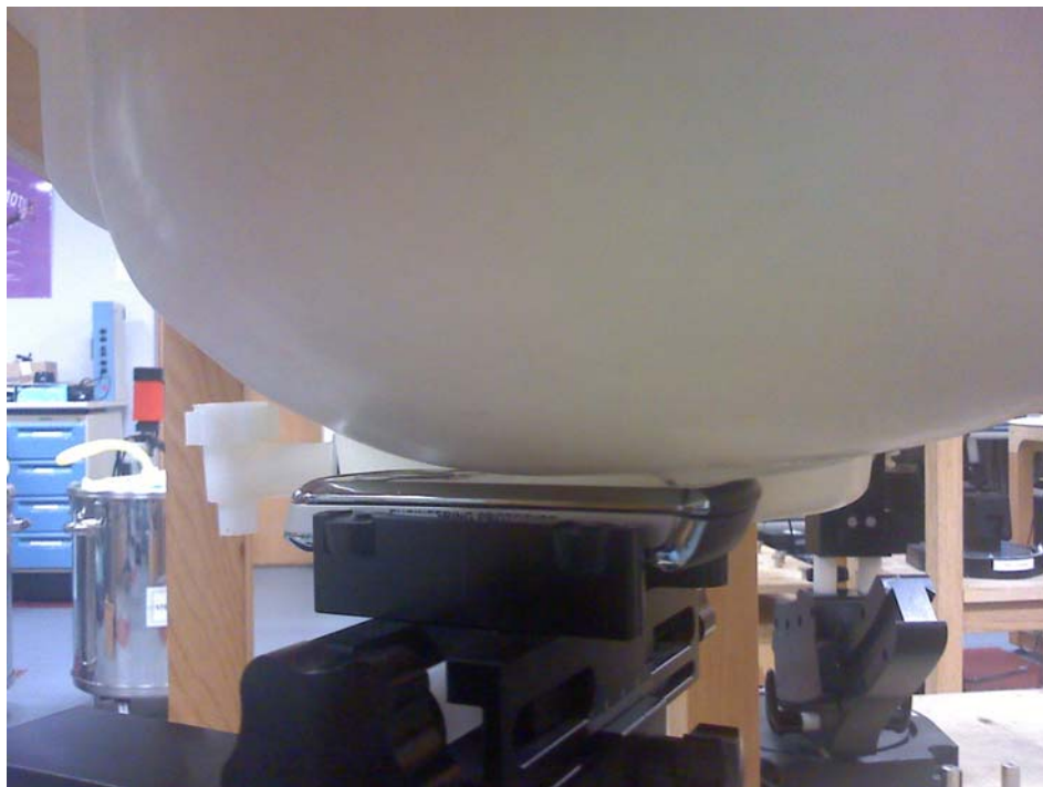
Figure 4 - Transceiver against head, Cheek Touch position – Slider Closed
