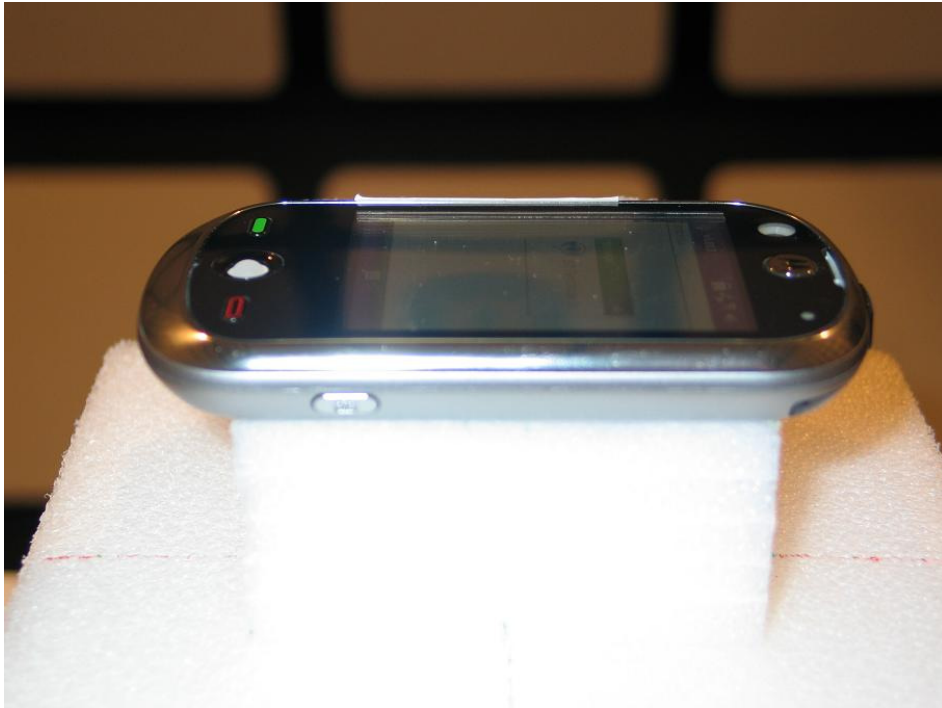
22298-1, IHDP56JH1 placed in test position X
