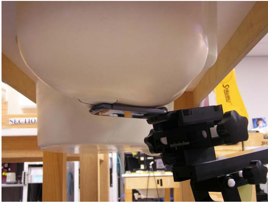
Figure 3 – Transceiver against head, Cheek Touch position
