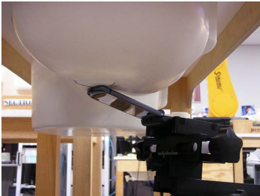
Figure 4 – Transceiver against head, 15° Tilt position
