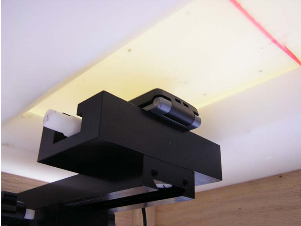
Figure 5 – Transceiver against body, Back of Phone 15 mm from Phantom position
