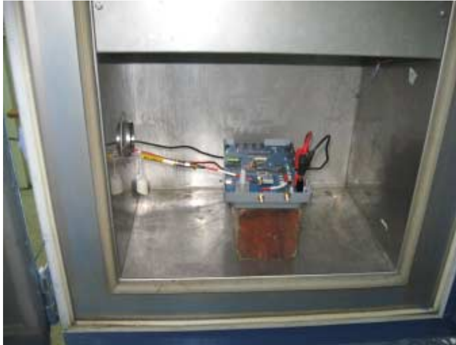
Photograph No.10 Setup for frequency stability measurements
