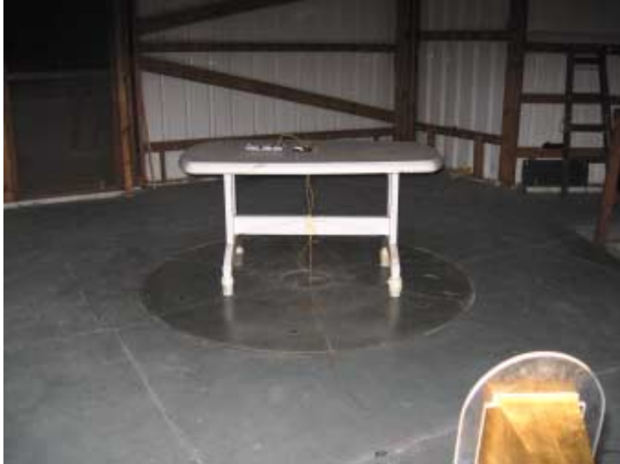
Photograph No.7 Spurious emissions measurement setup at the OATS
