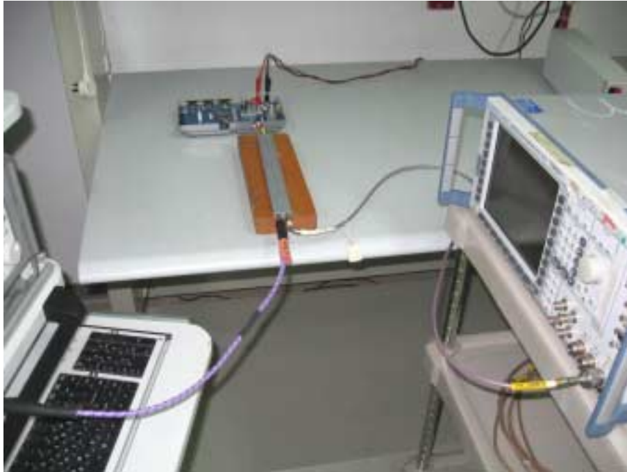
Photograph No.2 Spurious conducted emissions measurement setup
