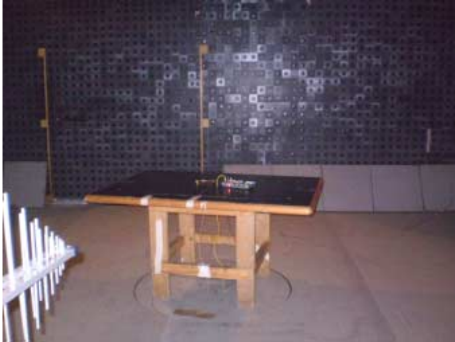
Photograph No.4 Spurious emissions measurement setup in the anechoic chamber with biconilog antenna
