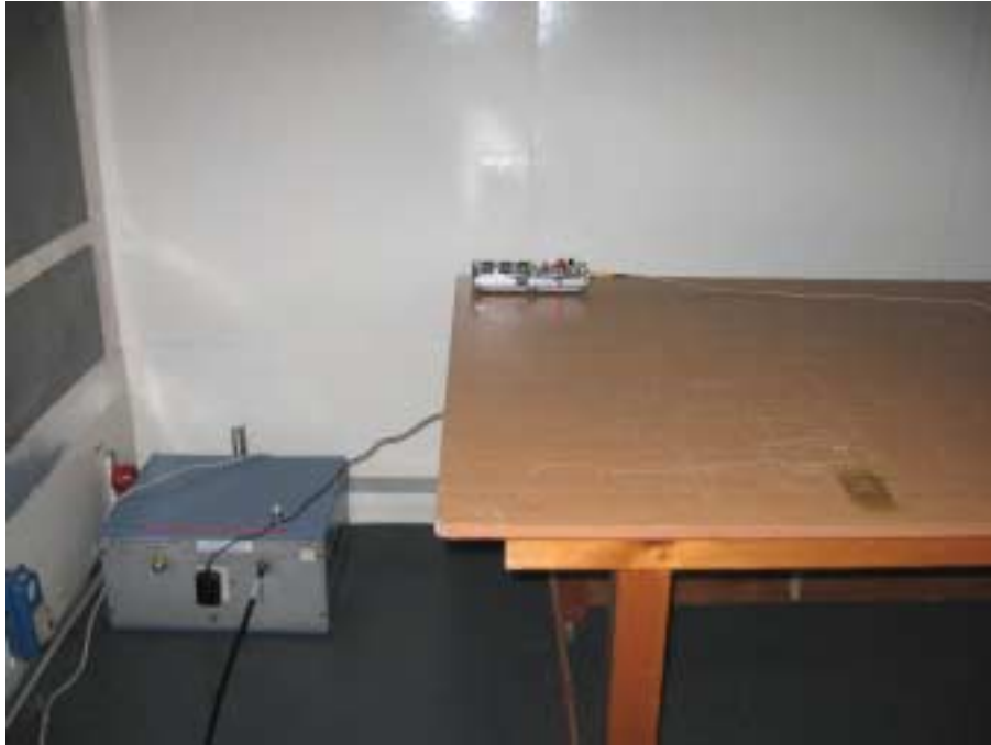
Photograph No.11 Setup for conducted emission measurements on the EUT power lines
