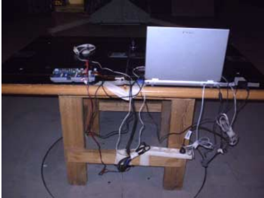
Photograph No.9 Radiated emission field strength measurements in the anechoic chamber, close view
