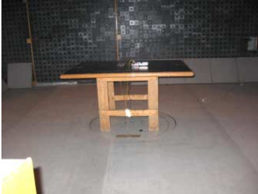
Photograph No.5 Spurious emissions measurement setup in the anechoic chamber with double ridge guide antenna
