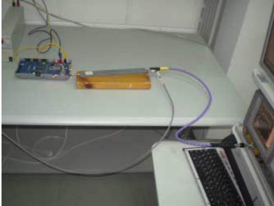
Photograph No.1 Peak output power, occupied bandwidth and receiver spurious conducted emissions measurement setup
