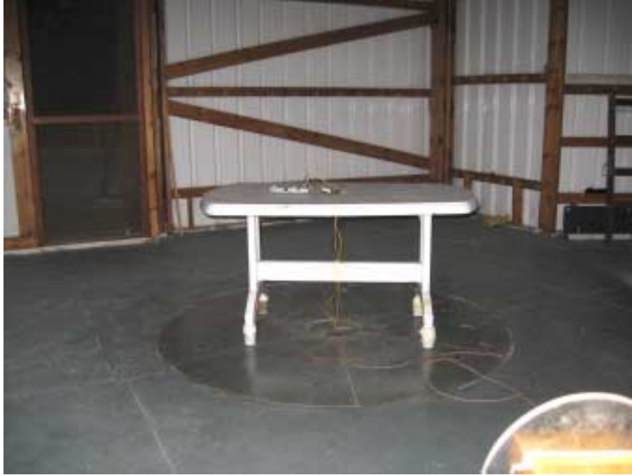
Photograph No.6 Spurious emissions measurement setup at the OATS
