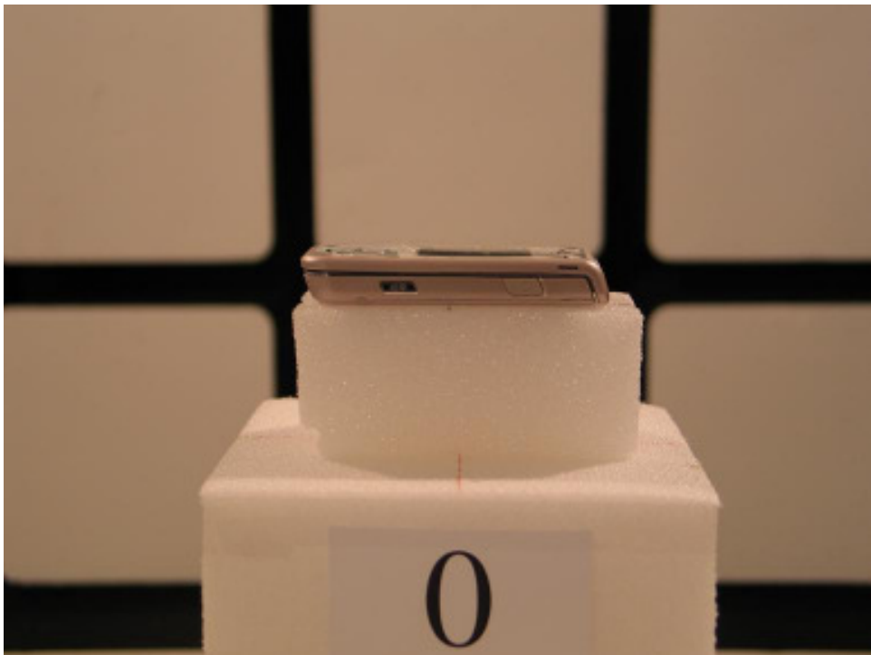
21780-1, IHDP56JD1 placed in test position X - Closed
