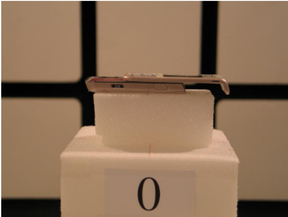
21780-1, IHDP56JD1 placed in test position X - Open
