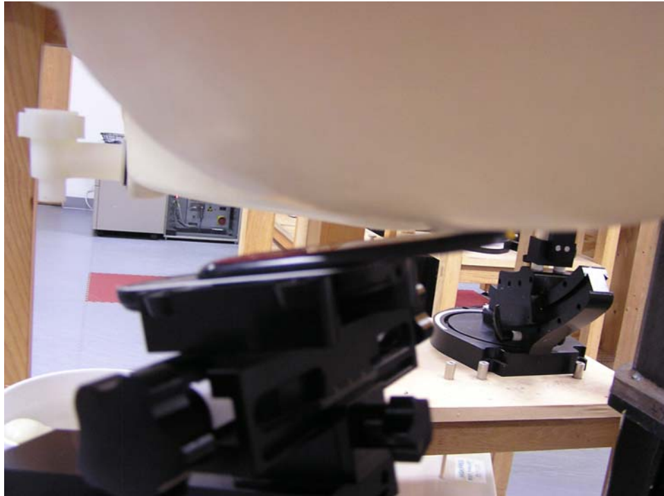
Figure 7 - Transceiver against head, 15° Tilt position – Slider Open
