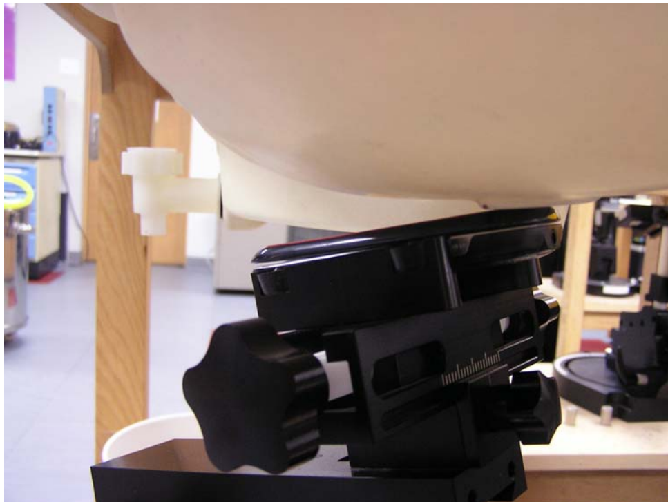
Figure 6 - Transceiver against head, 15° Tilt position – Slider Closed
