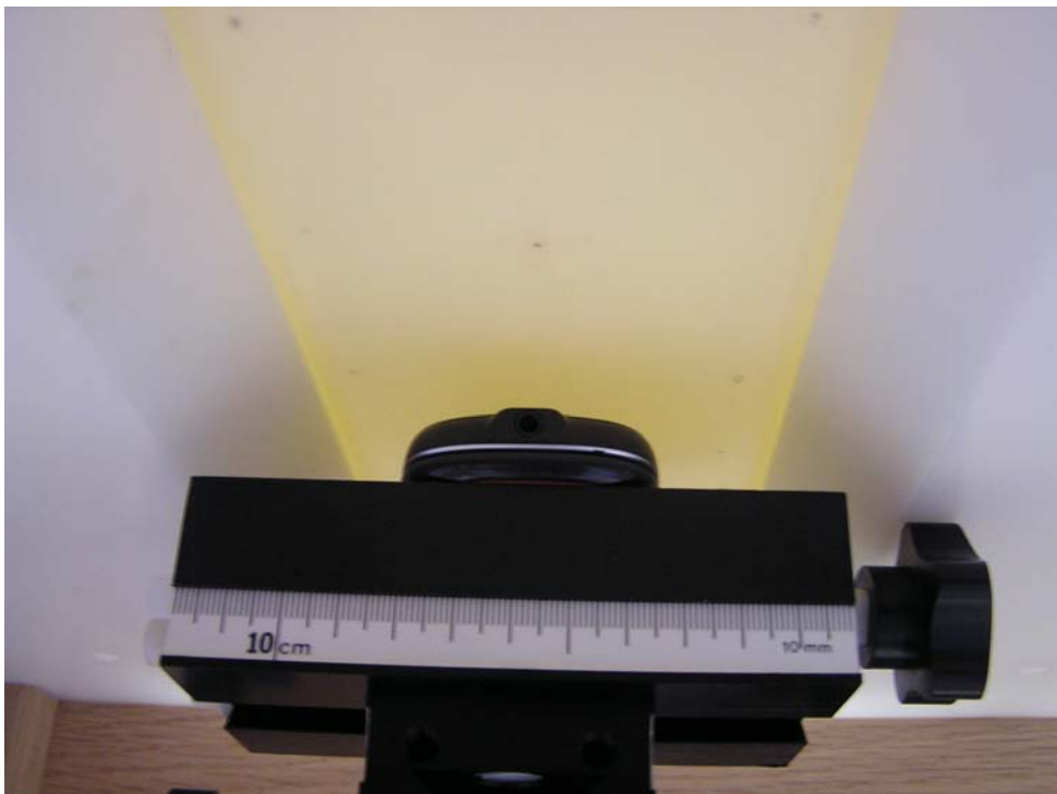
Figure 8 - Transceiver against body, 15 mm from Phantom position
