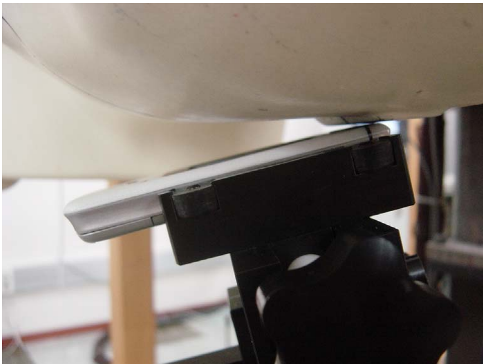
Figure 4: Phone Against the Head Phantom (15° Tilt)
