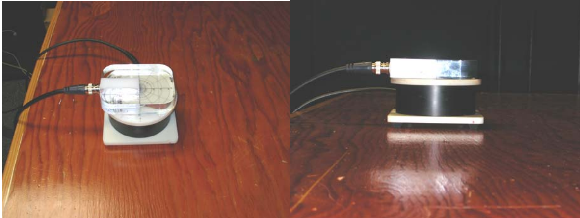
Figure 6-1 – Probe coil being calibrated with TMFS
