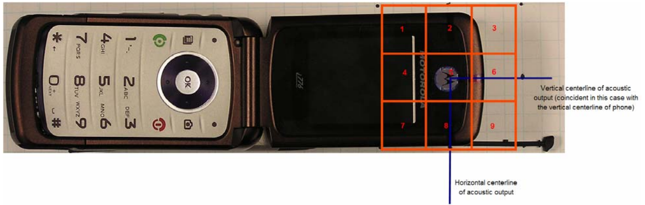
Figure 3. Phone Front - Orientation and Measurement Plane for RF Emissions Testing
