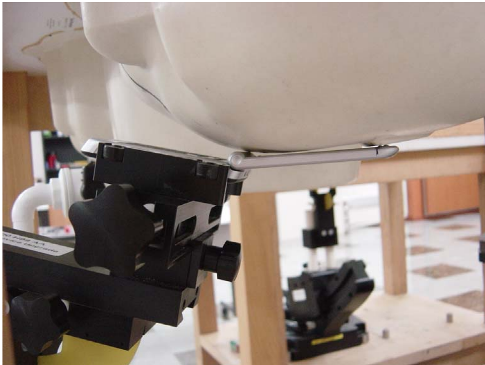
Figure4: Phone Against the Head Phantom (Cheek Touch)
