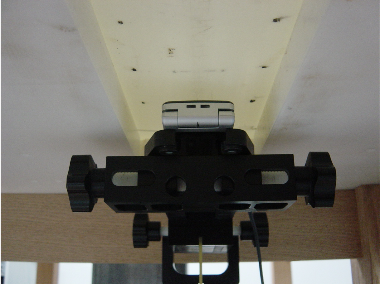
Figure6: Phone Against the Flat Phantom
