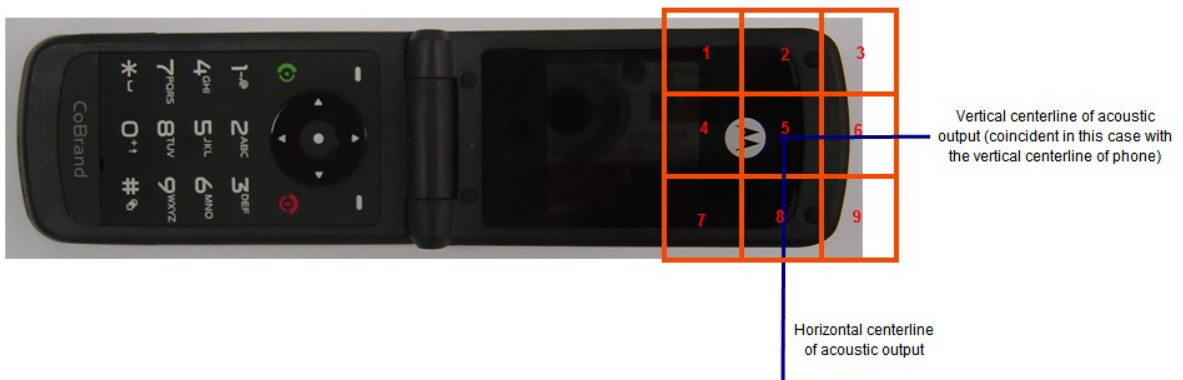
Figure A5-3. Phone Open - Orientation and Measurement Plane for RF Emissions Testing
