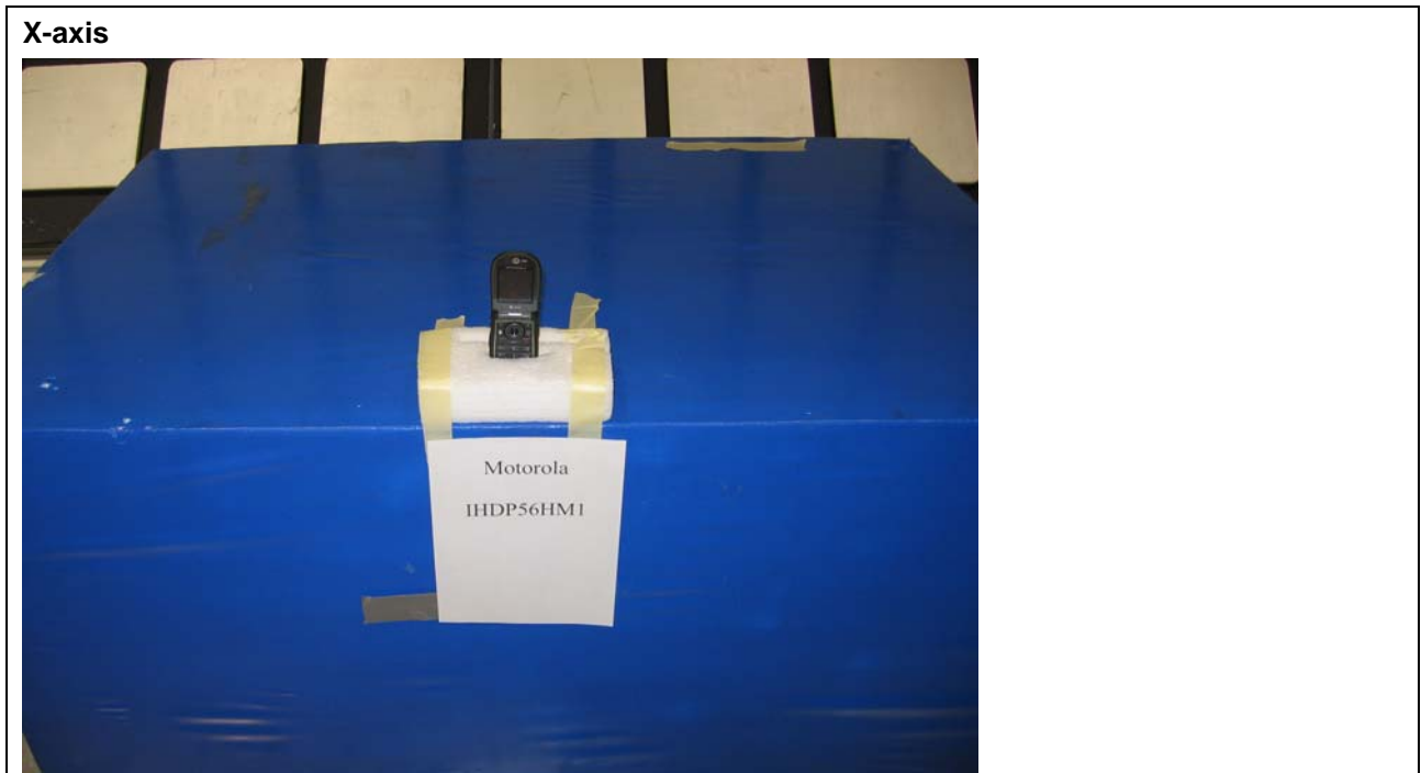
Figure 1 Test setup for Radiated Emissions
