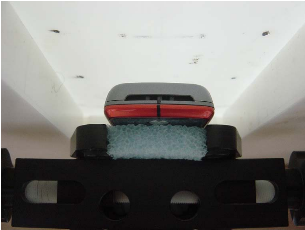
Figure5: Phone Against the Flat Phantom
