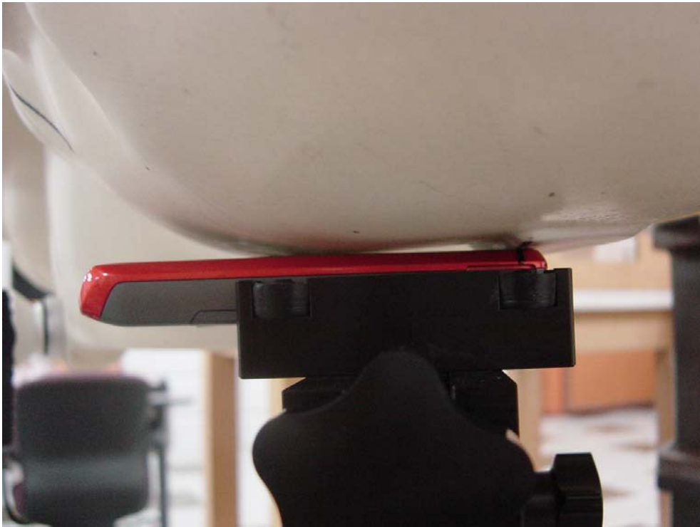
Figure3: Phone Against the Head Phantom (Cheek Touch)
