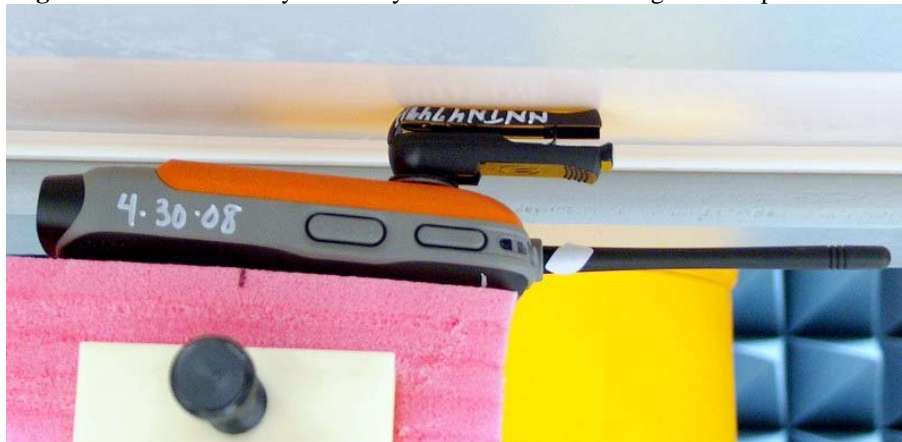
Figure 2: DUT with carry accessory model NNTN4747A against the phantom.
