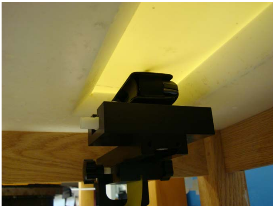
Figure 12. Body Worn Testing with Pouch
