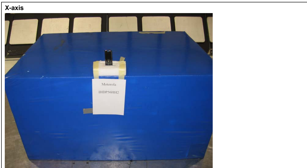
Figure 1 Test setup for Radiated Emissions
