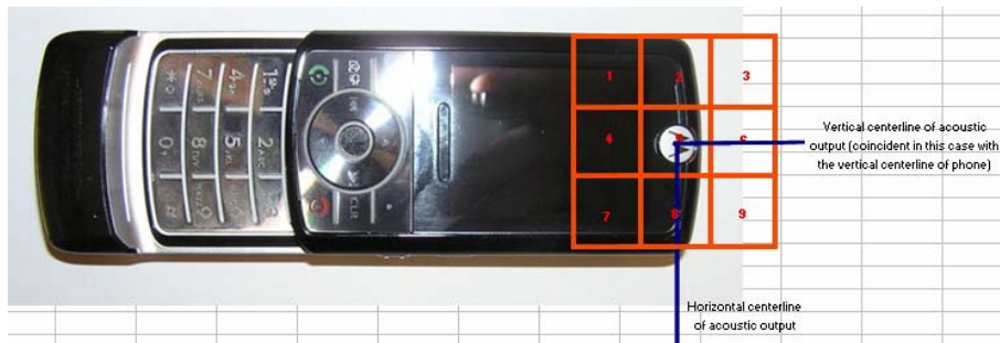
Figure A4-4. Location of Measured Points
