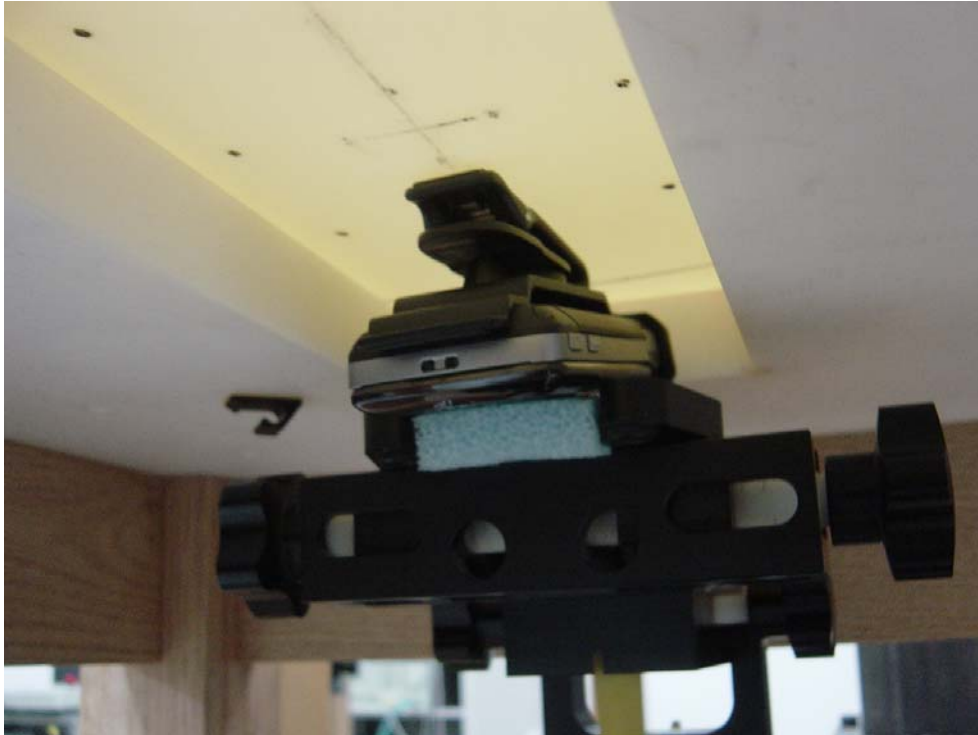
Figure 14: Phone Against the Flat Phantom with KAYN4103A Holster with Rotating Clip
