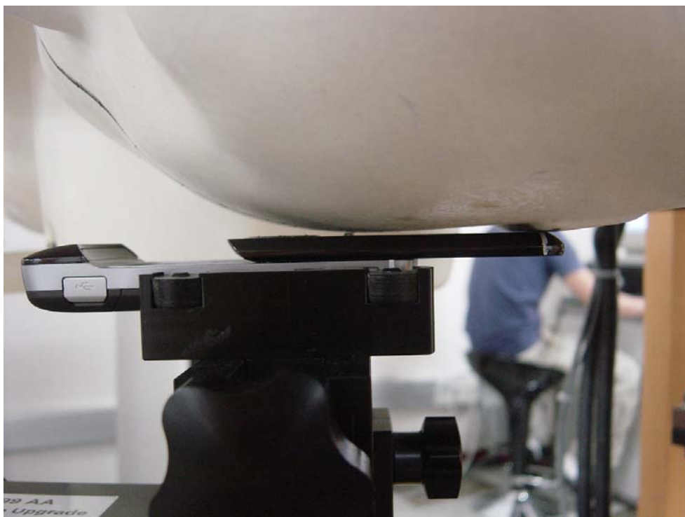
Figure 9. Phone Against the Head Phantom (Cheek Touch – Slider Up)
