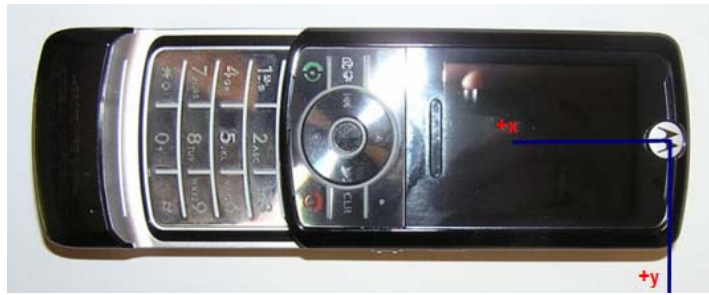
Figure A4-3. Coordinate Axis for T-coil Measurements
