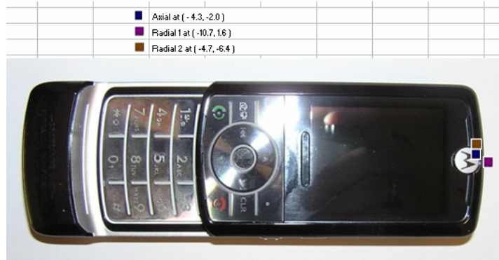
Figure A4-3. Coordinate Axis for T-coil Measurements
