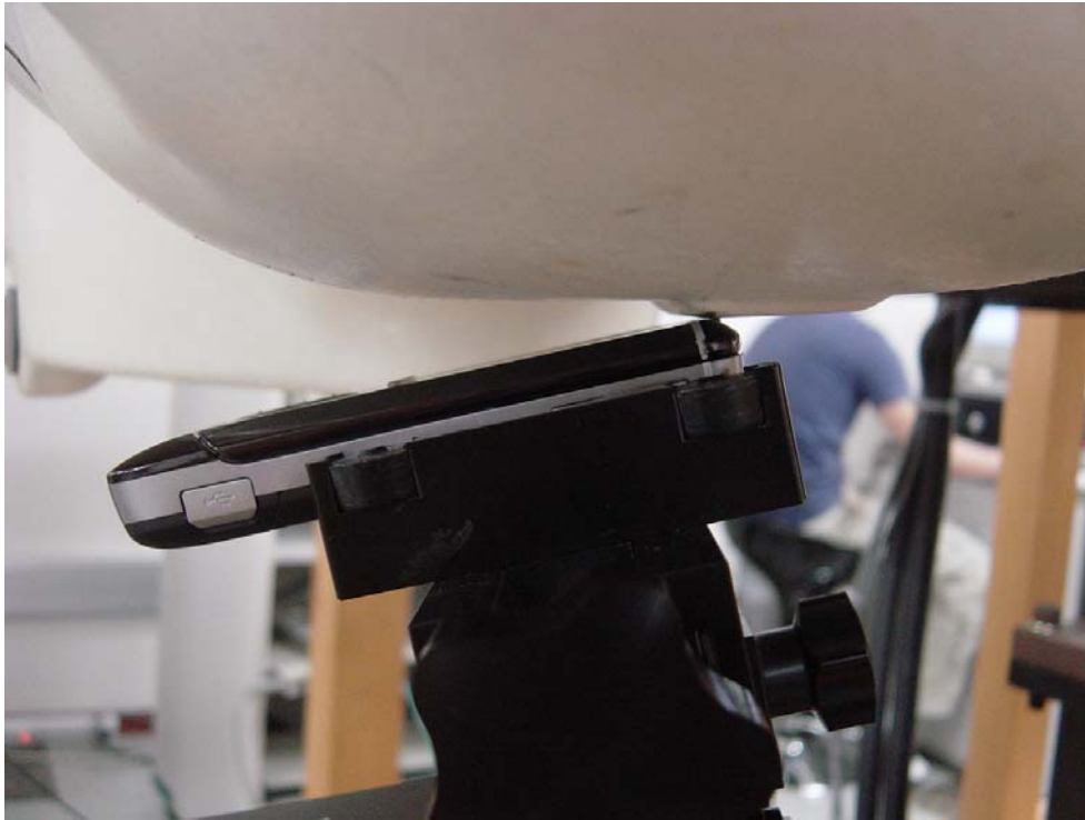
Figure 10. Phone Against the Head Phantom (15°Tilt – Slider Down)
