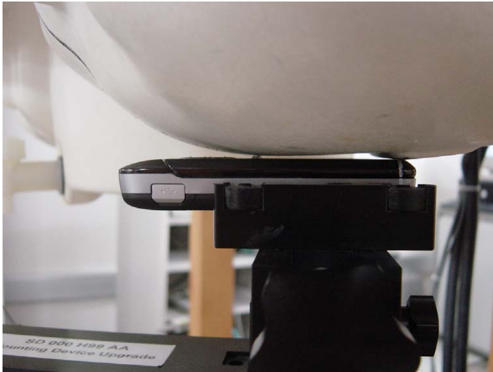
Figure 8. Phone Against the Head Phantom (Cheek Touch – Slider Down)
