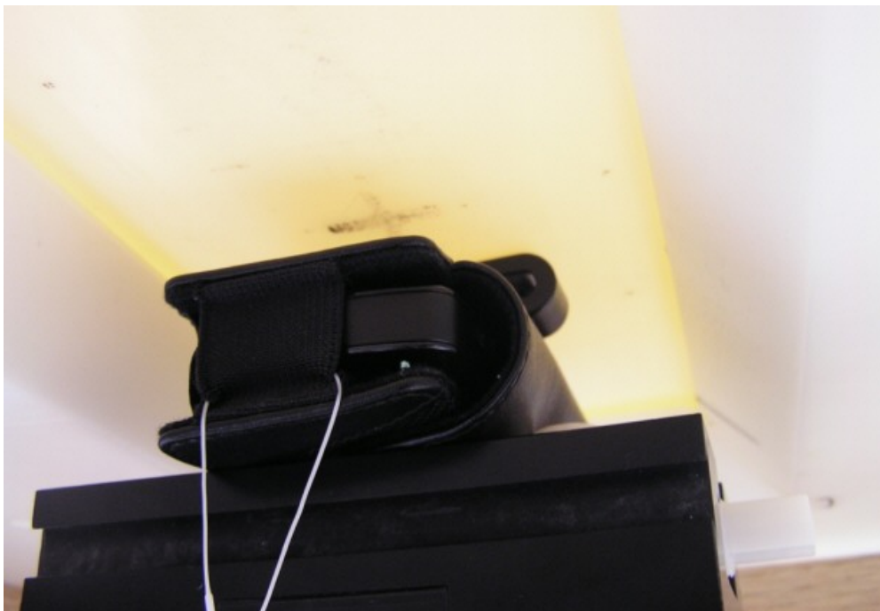
Figure 13: Phone Against the Flat Phantom in SYN1531A Case
