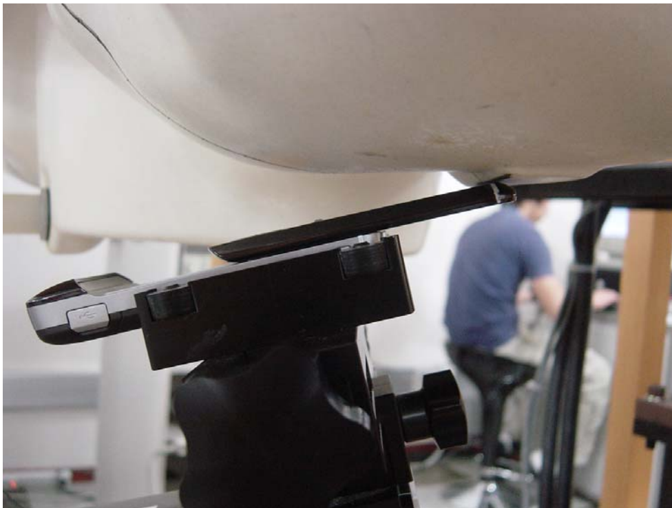
Figure 11. Phone Against the Head Phantom (15°Tilt – Slider Up)
