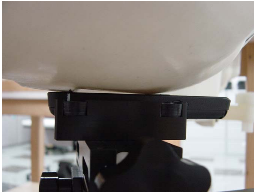
Figure 3 – Transceiver against head, Cheek Touch position
