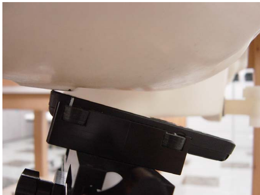
Figure 4 – Transceiver against head, 15° Tilt position
