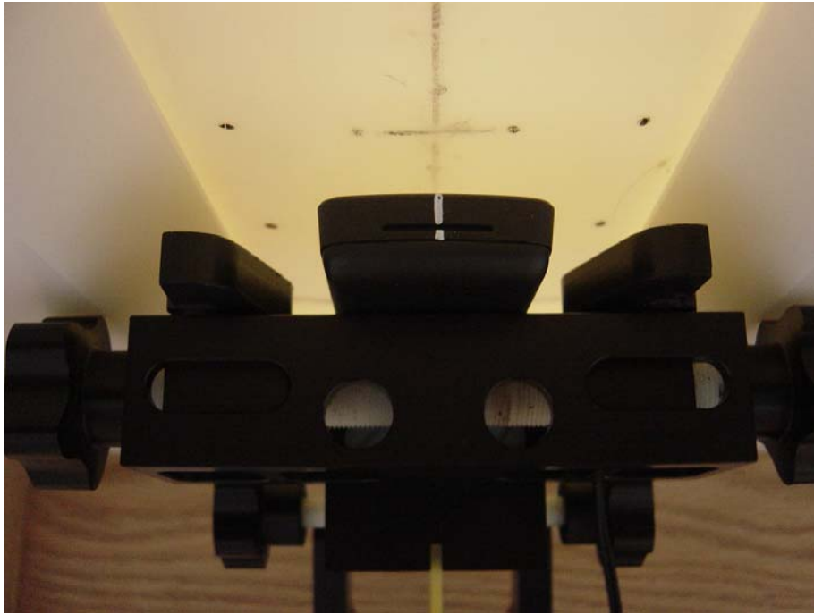
Figure 5 – Transceiver against body, Back of Phone 25 mm from Phantom position
