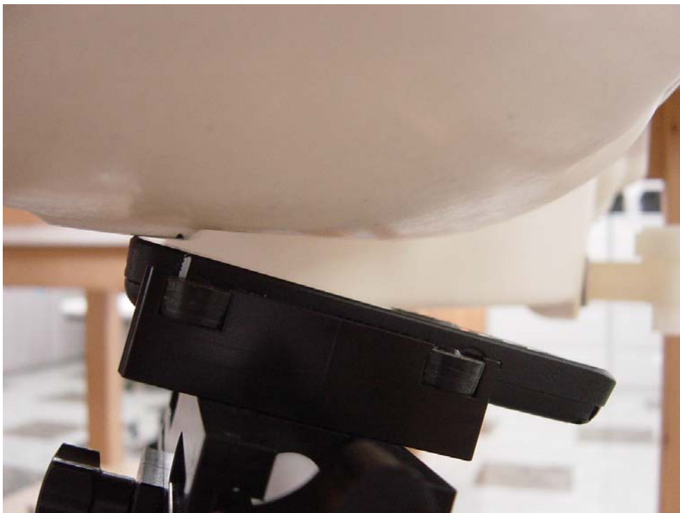
Figure4: Phone Against the Head Phantom (15° Tilt)
