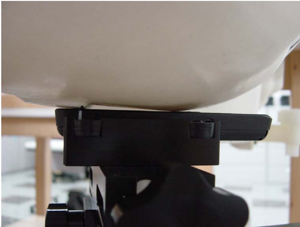
Figure3: Phone Against the Head Phantom (Cheek Touch)
