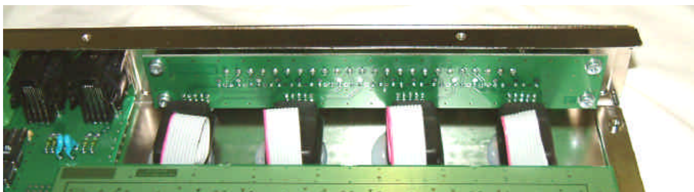
Detail view, cover removed (ES8mic – Terminal Block connectors board)
