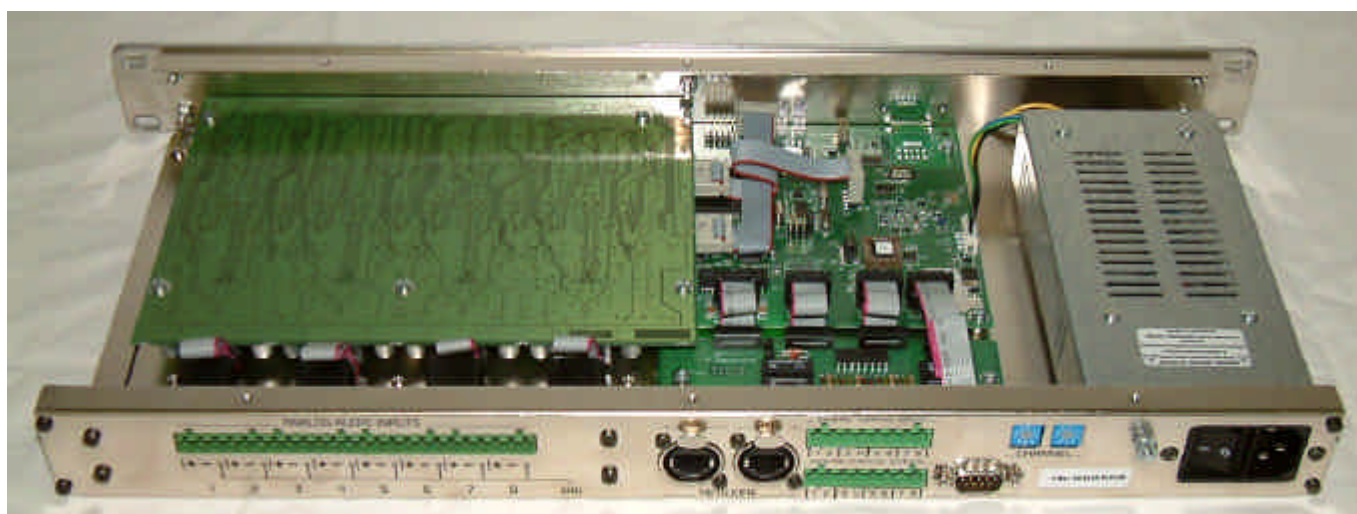
General view, cover removed, rear face (ES8mic- Terminal Block connectors)
