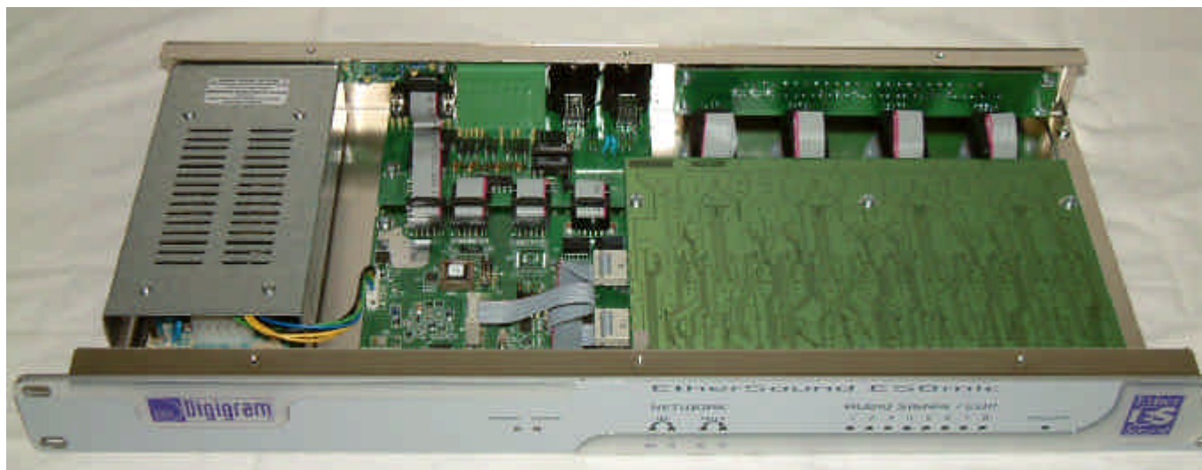
General view, cover removed, front face (ES8mic- Terminal Block connectors)
