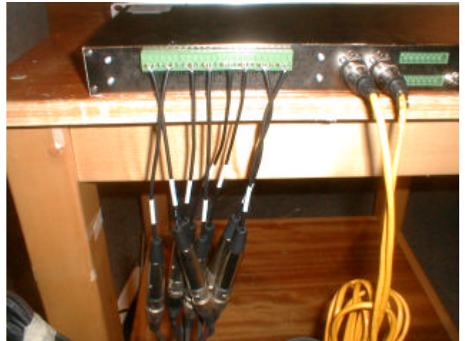
Detail view (XLR and terminal block connectors)
