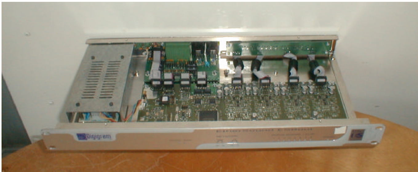
General view, cover removed, front face (ES8 IN & OUT – terminal block connectors)
