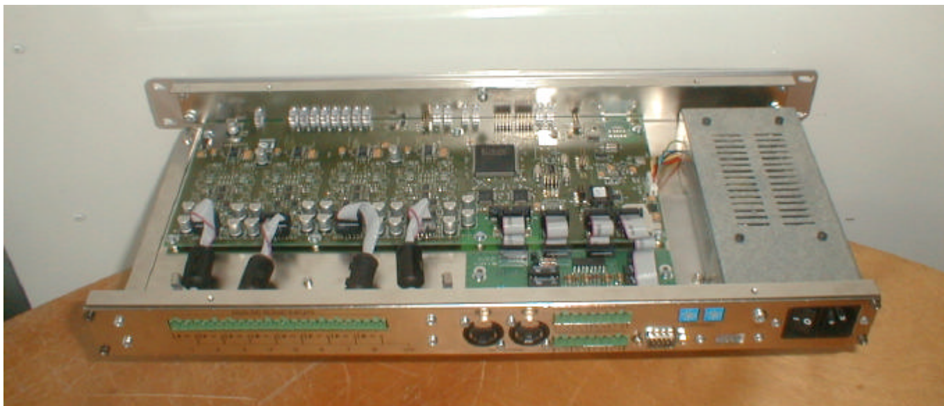
General view, cover removed, rear face (ES8 IN & OUT – terminal block connectors)
