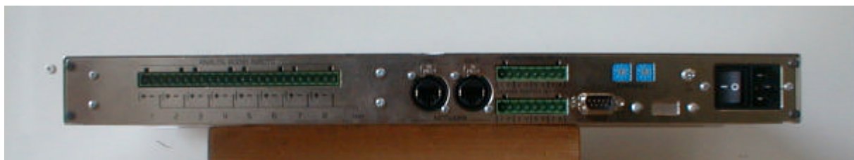
General view, rear side (ES8 OUT &IN – Terminal block connectors)
