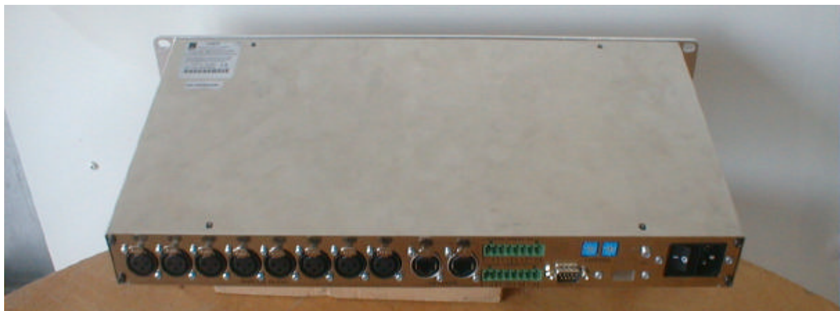
General view, rear side (ES8 OUT &IN – XLR connectors)
