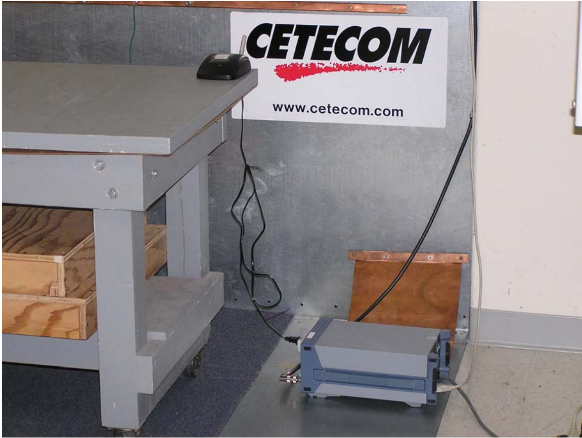
Test setup – AC Line Conducted Emissions
