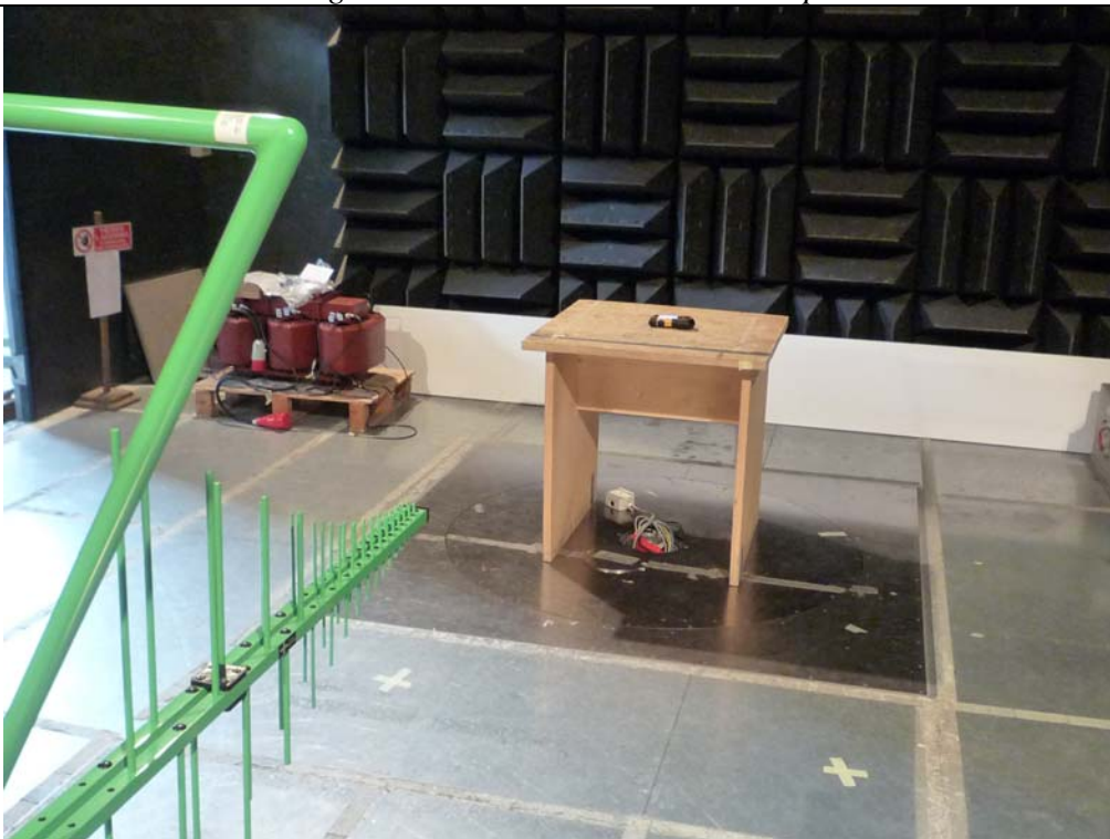
Fig. 2 Radiated emission test set-up
