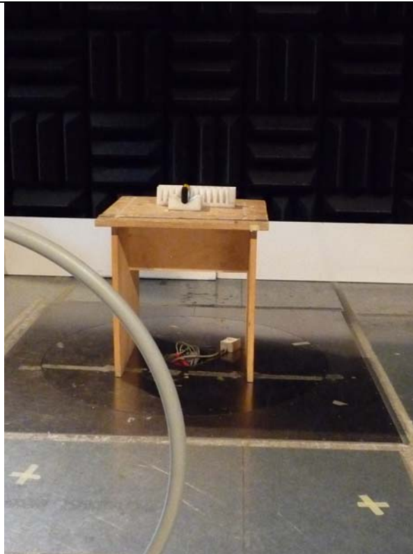
Fig. 1 Radiated emission test set-up
