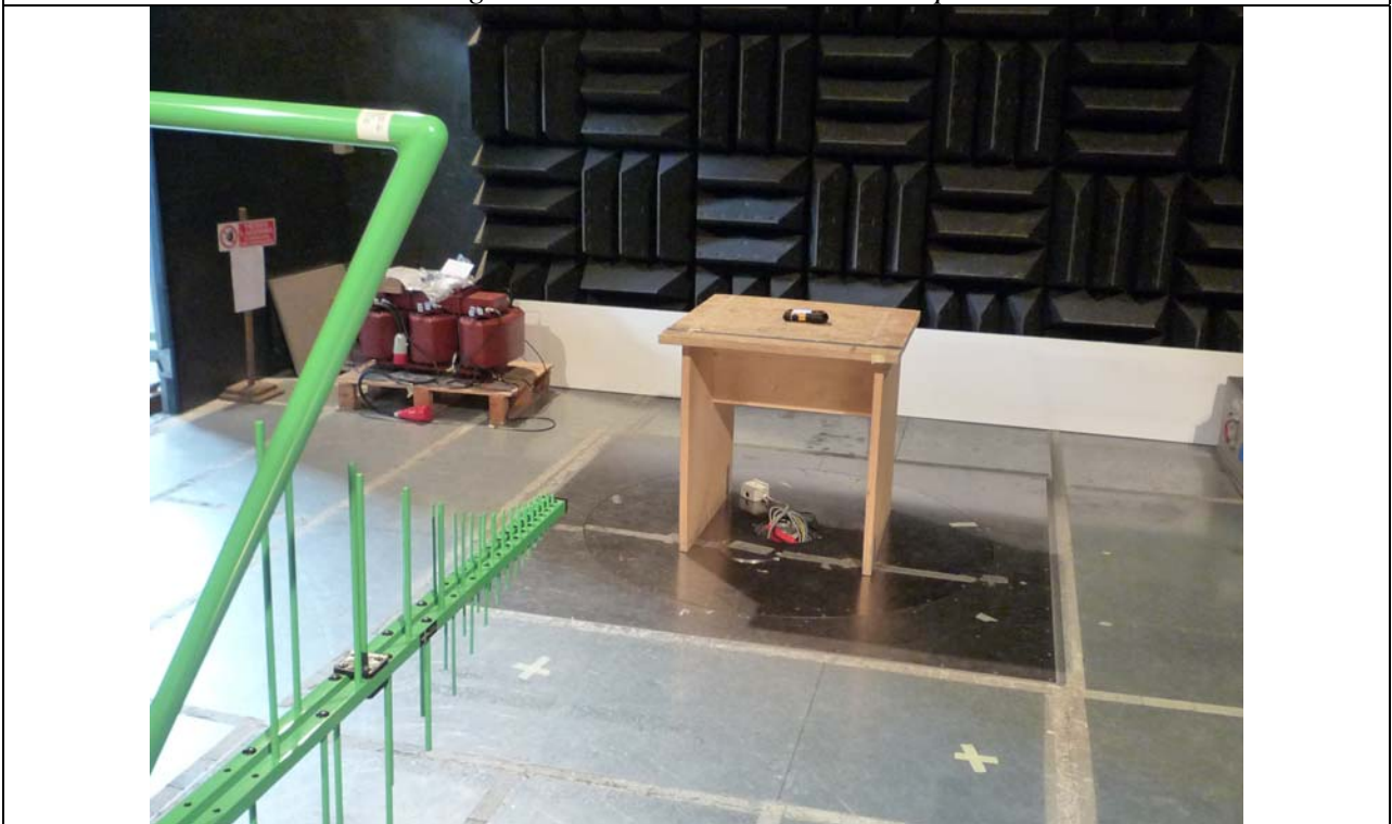
Fig. 8 Radiated emission test set-up
