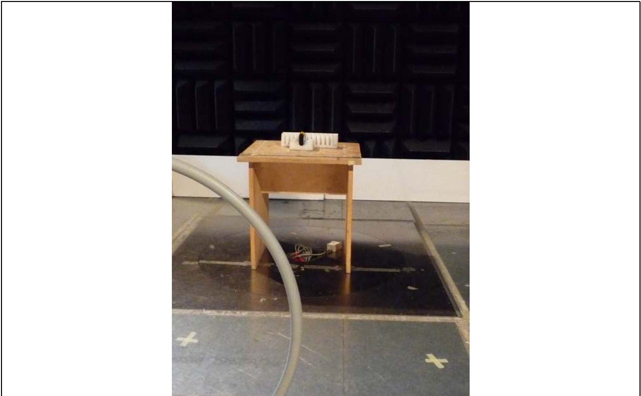
Fig. 7 Radiated emission test set-up
