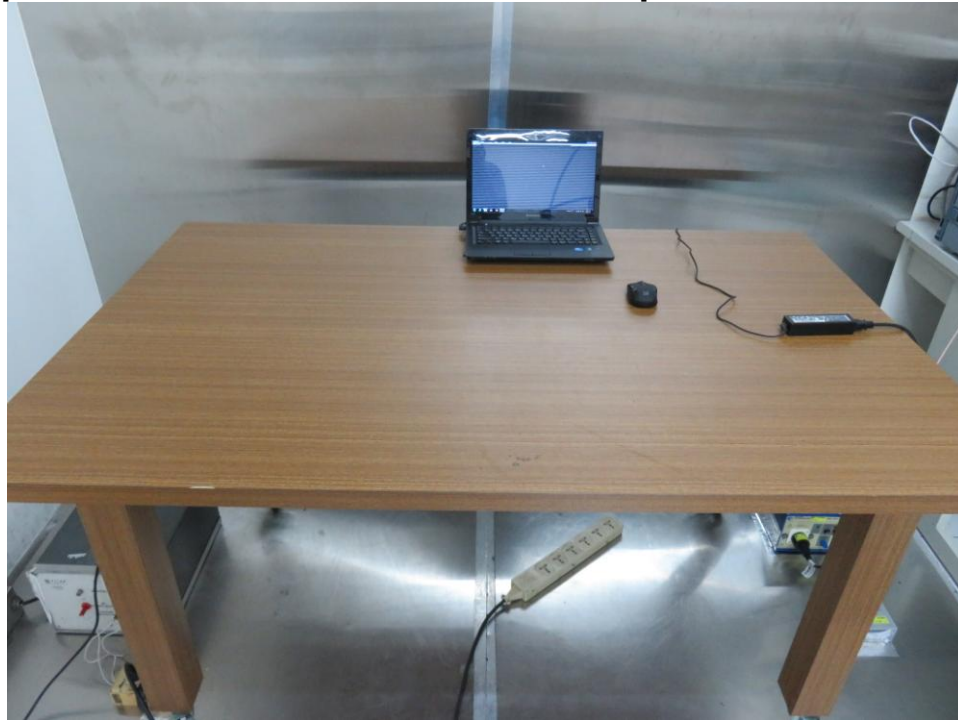
Photograph – Conducted Emission Test Setup
