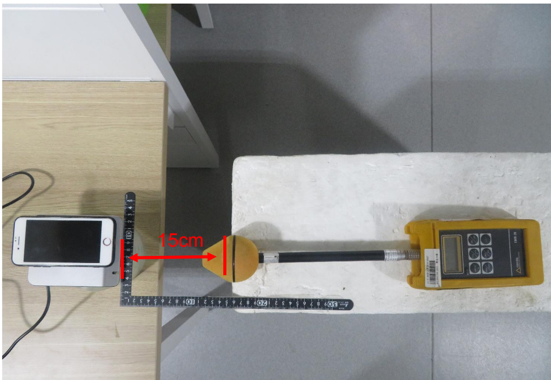
Description: RF Exposure Test Setup (Rear Side: 15cm)
