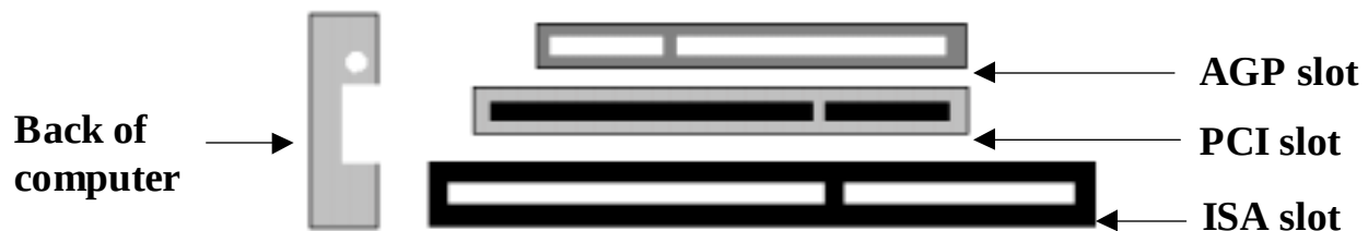
AGP vs. PCI vs. ISA expansion slots
