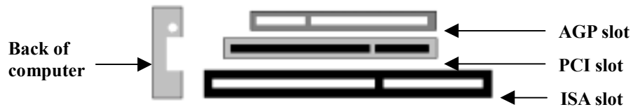
AGP vs. PCI vs. ISA expansion slots
