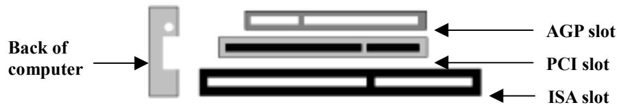
AGP vs. PCI vs. ISA expansion slots
