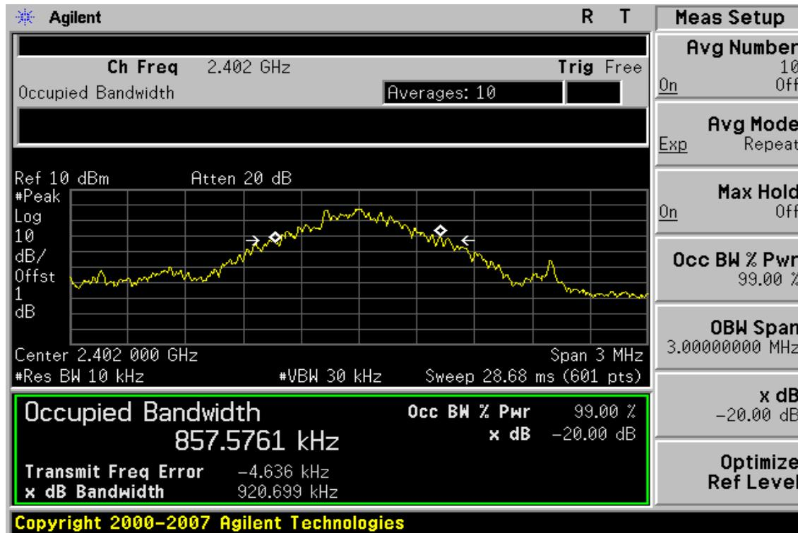
**20dB Bandwidth Test Data CH-Mid**
