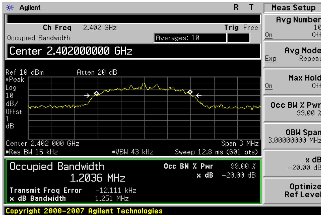
**20dB Bandwidth Test Data CH-Mid**
