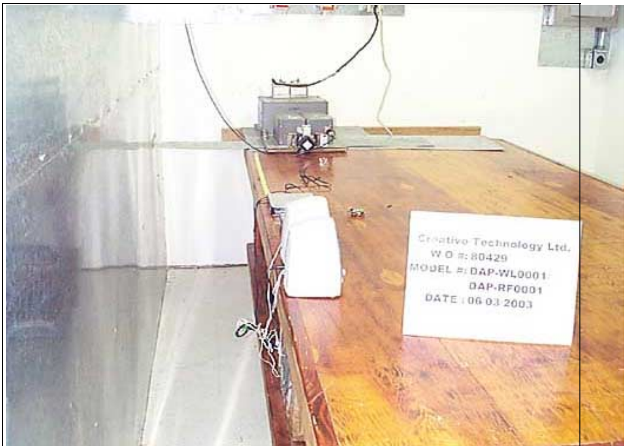
Mains Conducted Emissions - Side View
