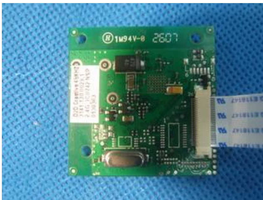
Fig. 5 –79 RF Module bottom view
