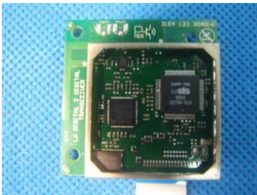
Fig. 6 – 79 RF Module shield removed view
