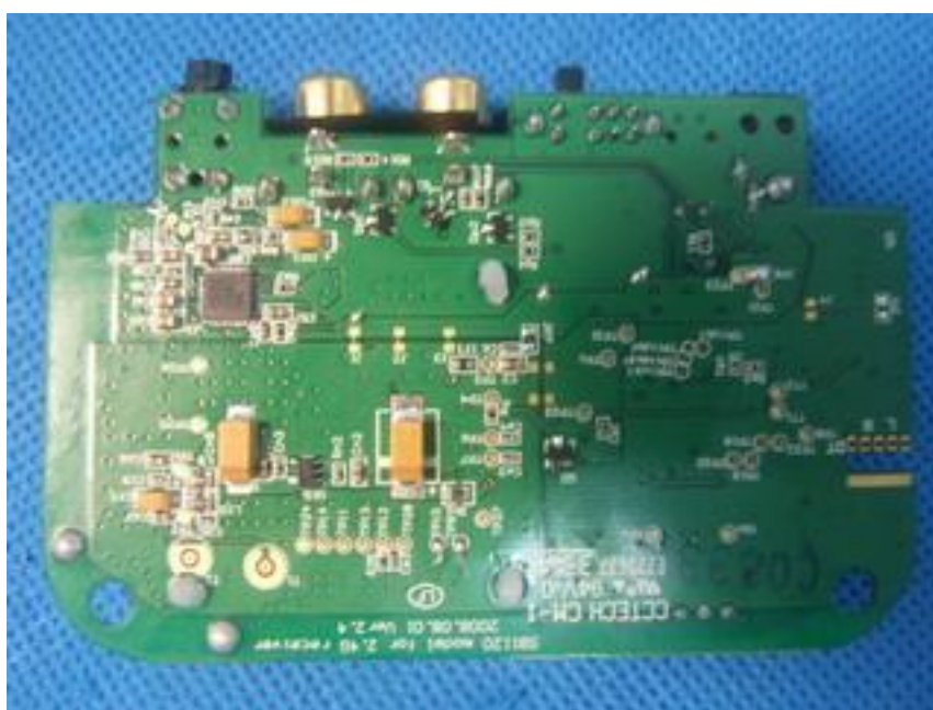
Fig. 5 –80 RF Module bottom view
