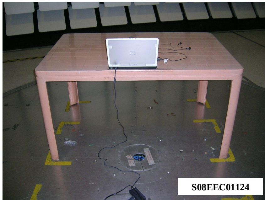
Radiated Emissions Test Setup (Rear View)
