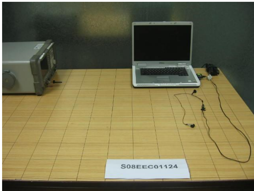
Conducted Emissions Test Setup (Front View)
