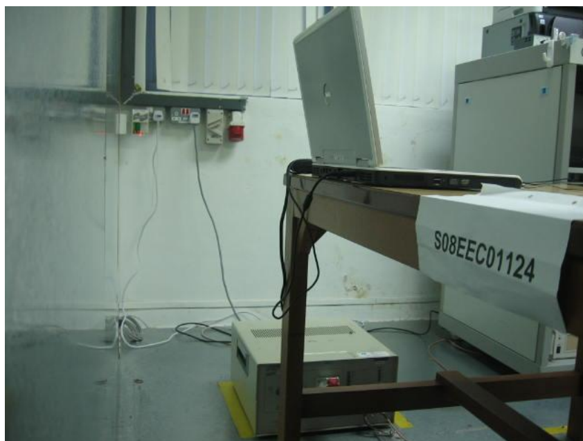
Conducted Emissions Test Setup (Rear View)
