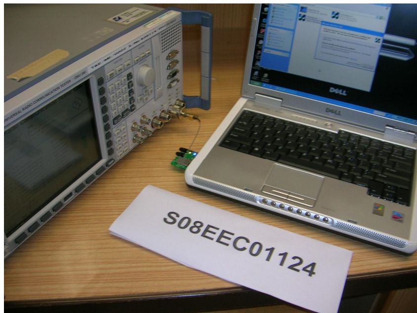
Maximum Peak Power Test Setup
