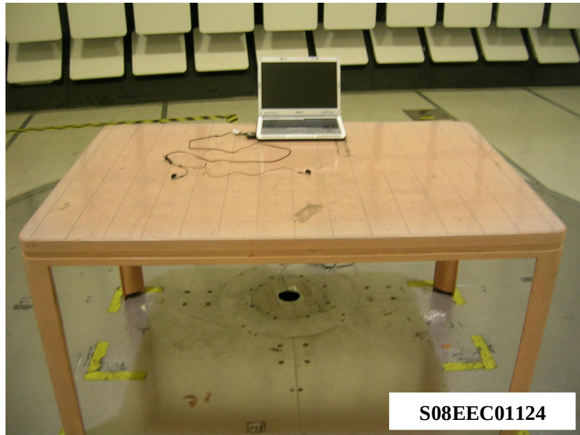
Radiated Emissions Test Setup (Front View)
