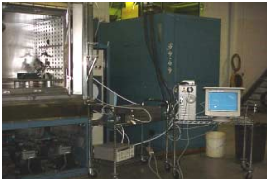
Figure 2-3. Typical overall test setup for damp heat functional test.
