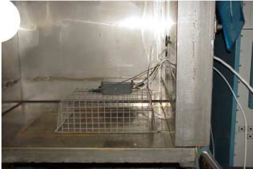
Figure 1-2. Typical chamber test setup for dry heat functional test.
