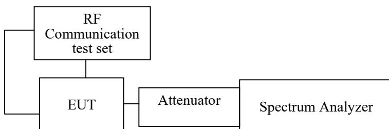
The OBW is the frequency bandwidth such that, below its lower and above its upper frequency limits, the mean powers are each equal to 0.5% of the total mean power of the given emission.
