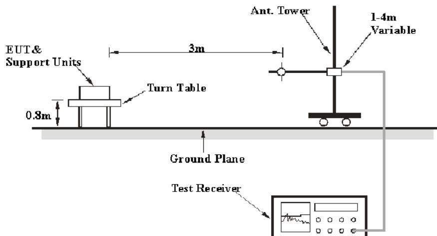
The radiated emission tests were performed in the 3 meters, using the setup accordance with the ANSI C63.10-2020. The specification used was the FCC Part 15.205 and 15.209 and 15.235 limits.
