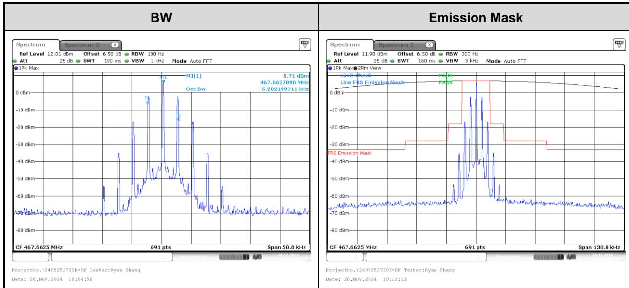
Note: unwanted emission for removed from the channel center frequency by more than 31.25kHz range, was required to measured with a reference bandwidth of at least 30 kHz, the factor for convert to 300Hz RBW is  $10 \times \log(30\text{kHz}/300\text{Hz}) = 20\text{dB}$ , the plot was measured using a 300Hz RBW and the result of this range was below the limit more than 20dB, so it would compliance the limit.
