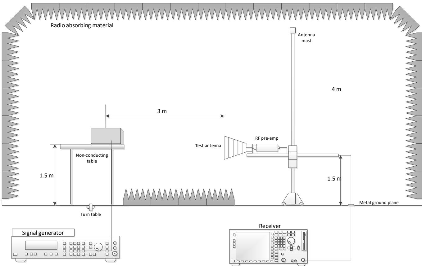
Figure 3.4-1: Test setup diagram
