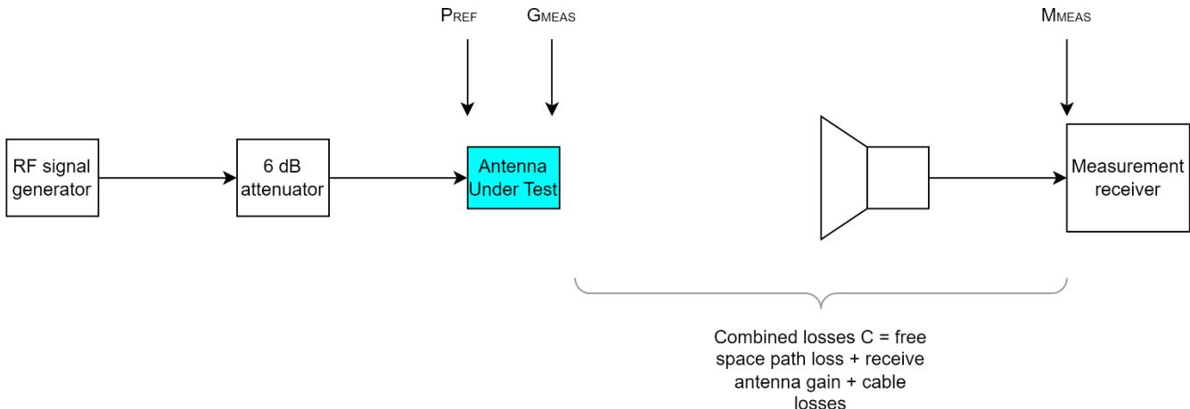
The peak received signal level at the measurement receiver is identified and noted as  $M_{MEAS}$ .
