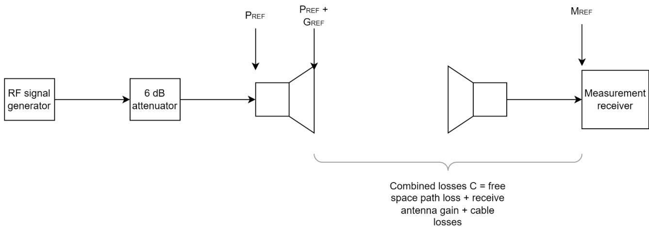
The signal level at the measurement receiver,  $M_{REF}$ , is recorded for each of the frequencies under test. Given that the transmit antenna is calibrated with a known gain  $G_{REF}$ , the following expression holds true:
