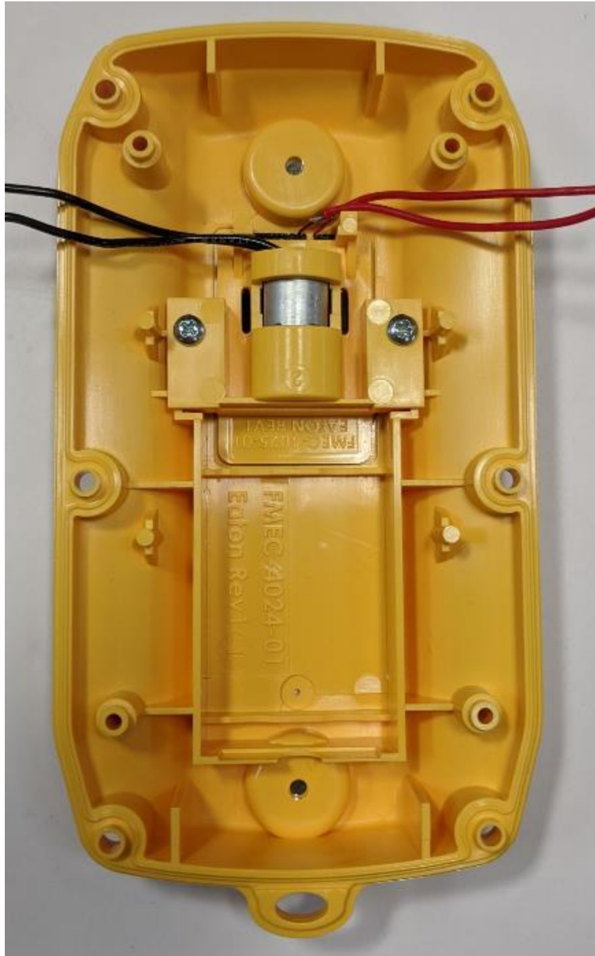
Figure 4 TD110 Back Shell Assembly.
