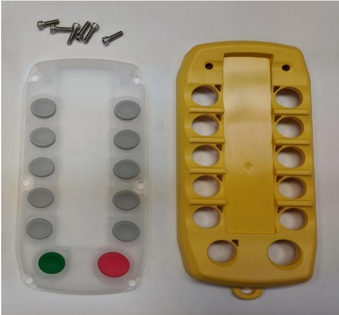
Figure 5 TD110 Front Shell Assembly.
