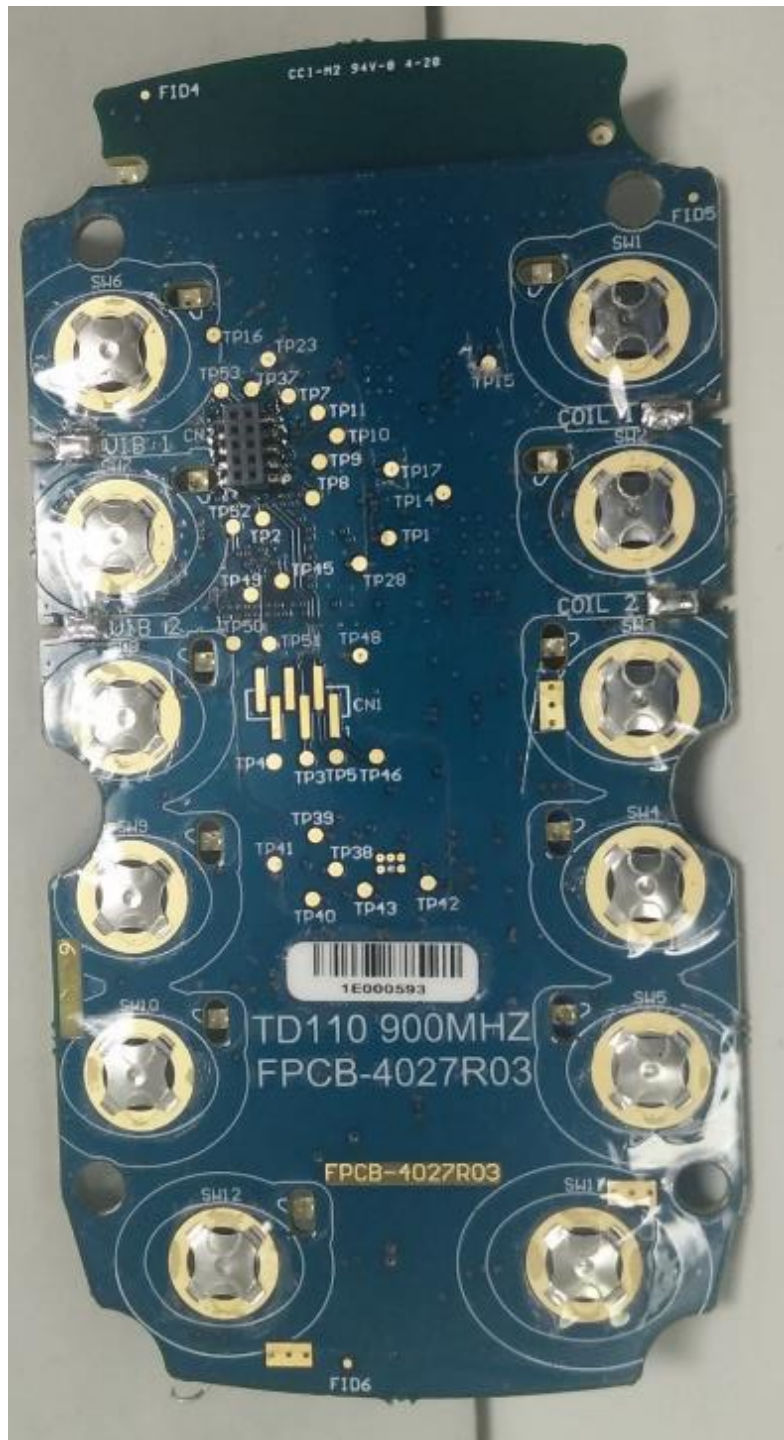
Figure 1 TD110 PCB top view with key domes installed.
