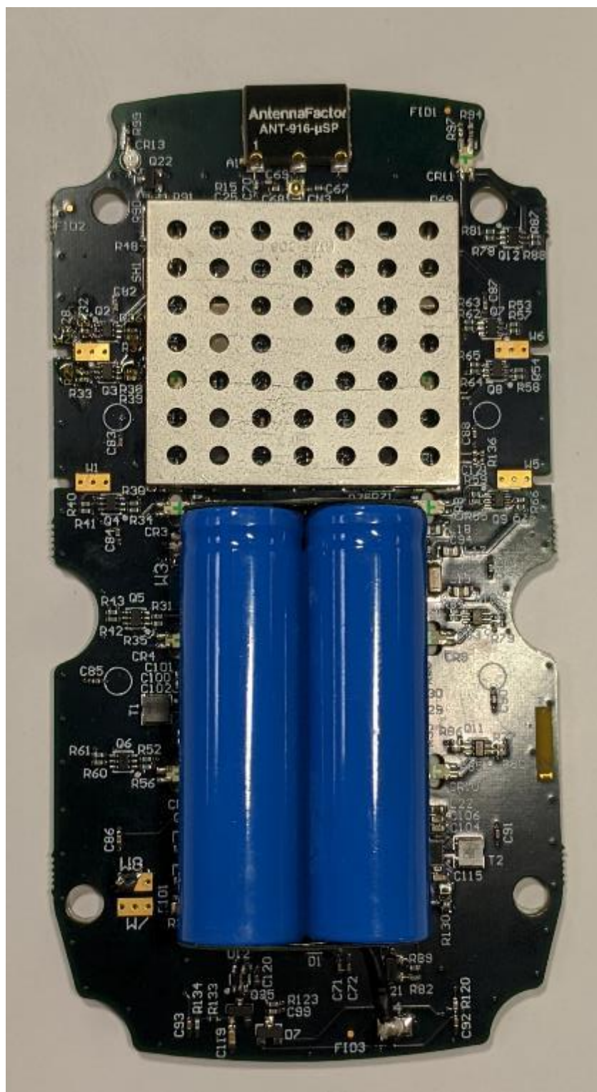
Figure 2 TD110 PCB bottom with battery and RF shield installed.
