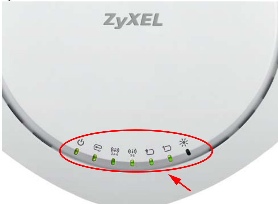
Figure 5 WAC6500 Series LEDs
