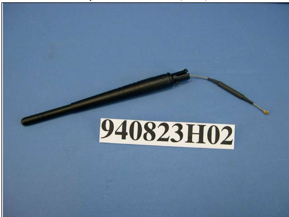
Dipole antenna <fix cable (8.3cm)>
