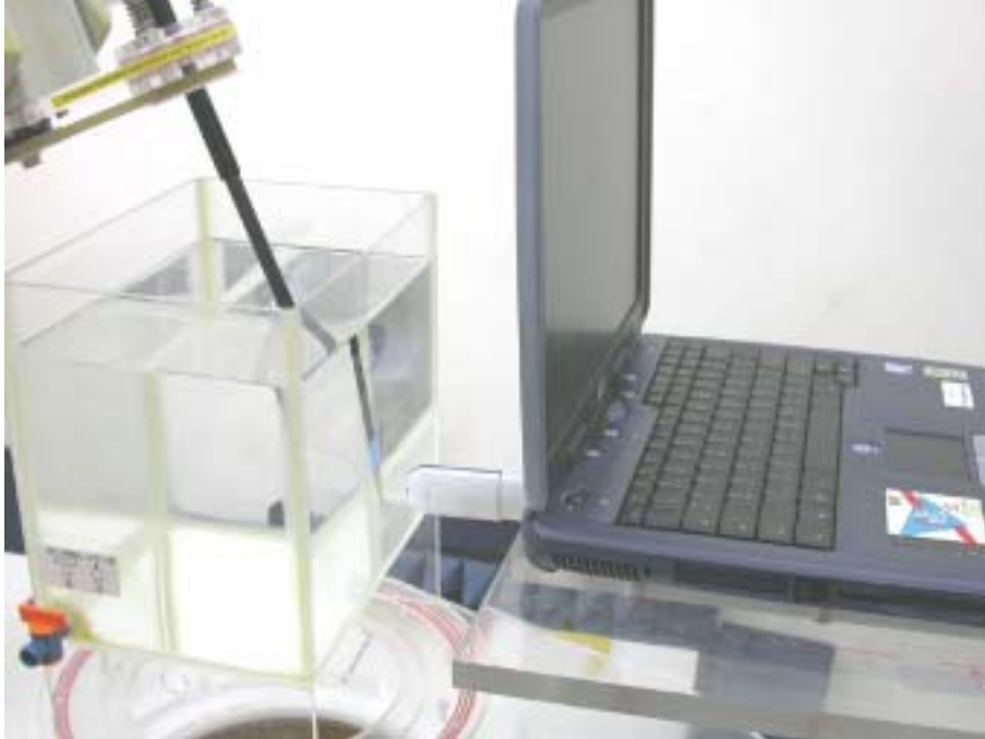
Figure 12: EUT perpendicular to phantom, 15 mm separation
