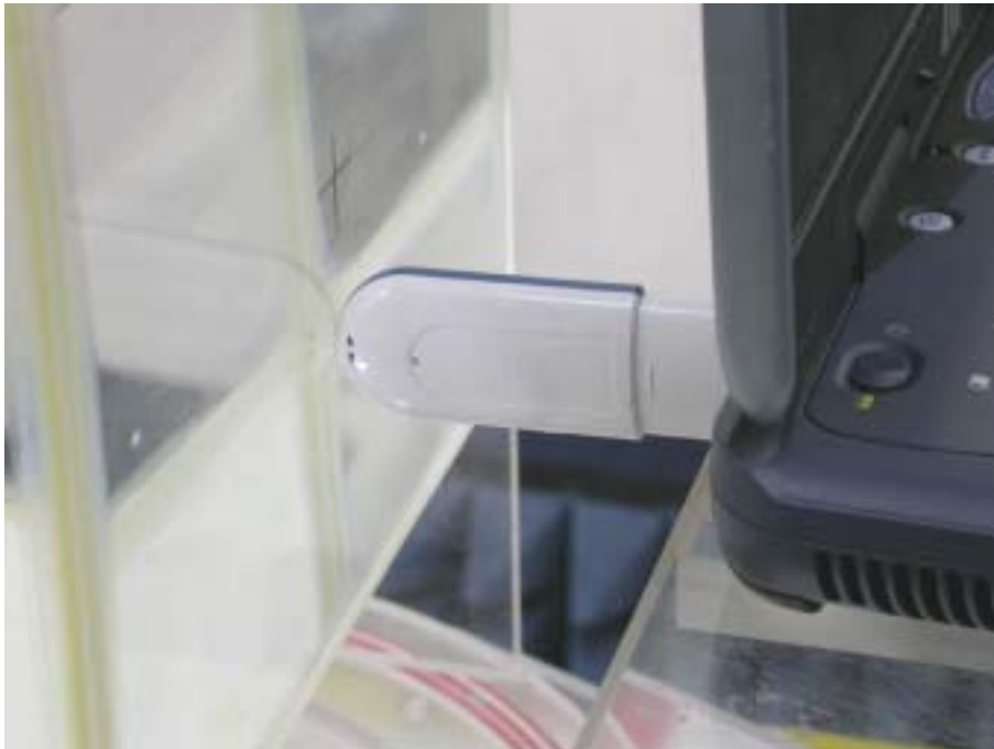
Figure 11: EUT perpendicular to phantom, 0 mm separation- Zoom In
