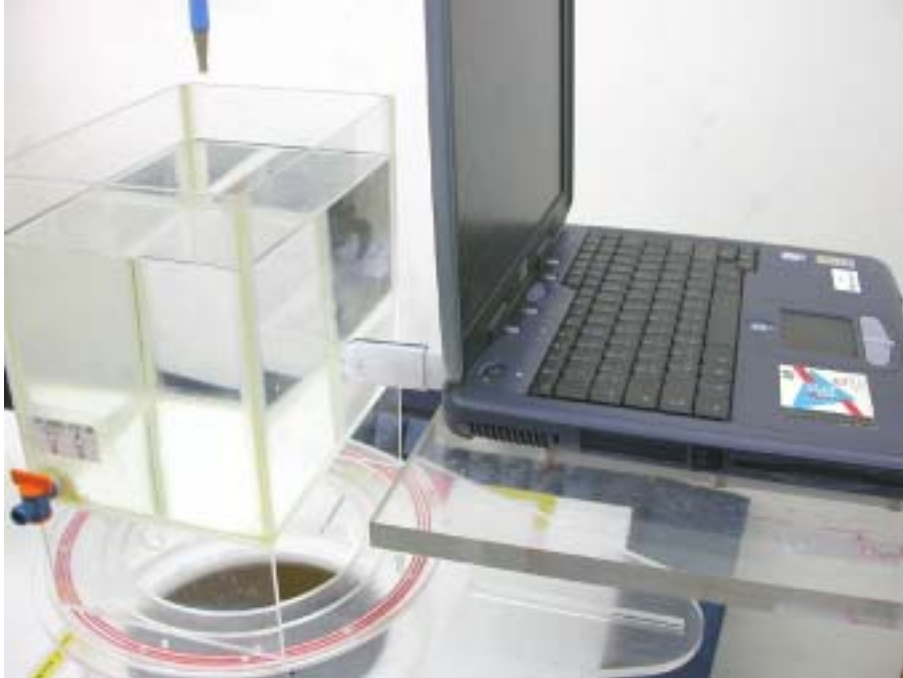
Figure 10: EUT perpendicular to phantom, 0 mm separation
