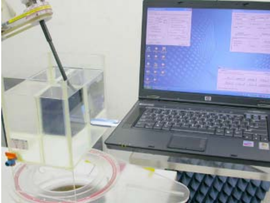
Figure 16: EUT perpendicular to phantom, 0 mm separation
