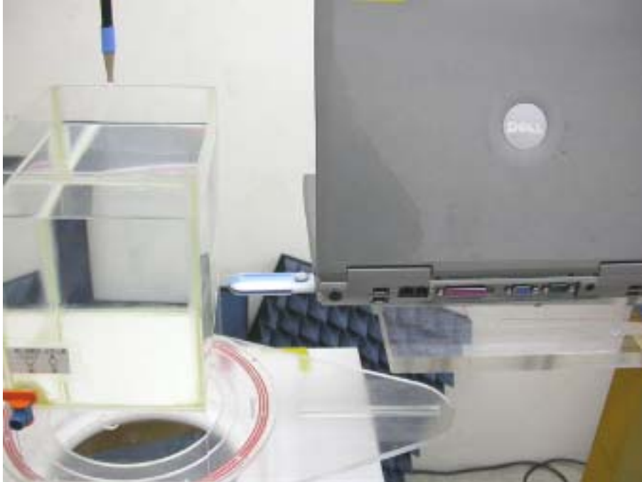
Figure 6: EUT perpendicular to phantom, 15 mm separation
