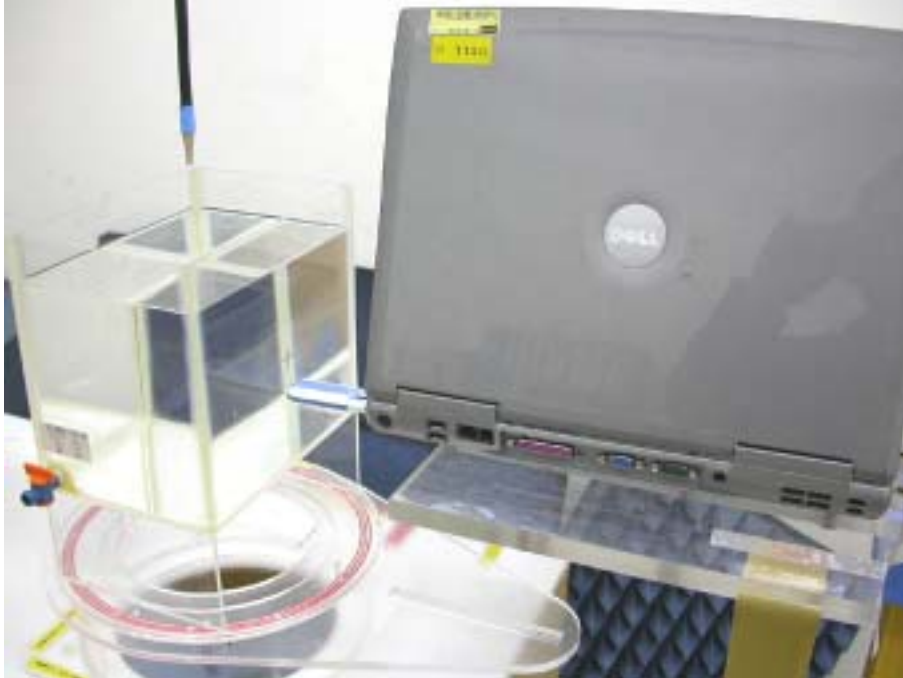
Figure 4: EUT perpendicular to phantom, 0 mm separation
