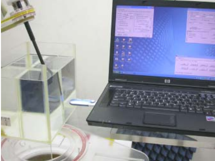
Figure 18: EUT perpendicular to phantom, 15 mm separation
