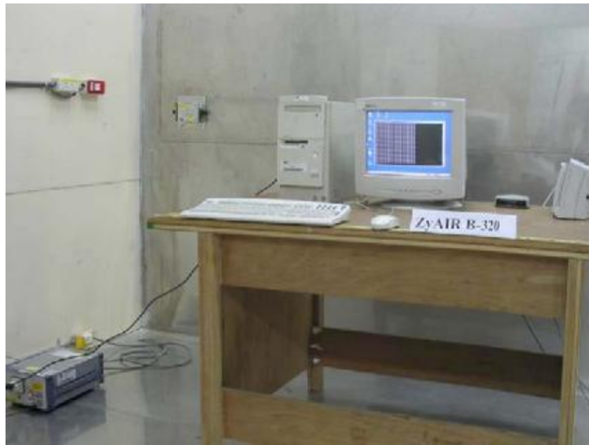
Photo 2: Conducted Emission Test Set-up
